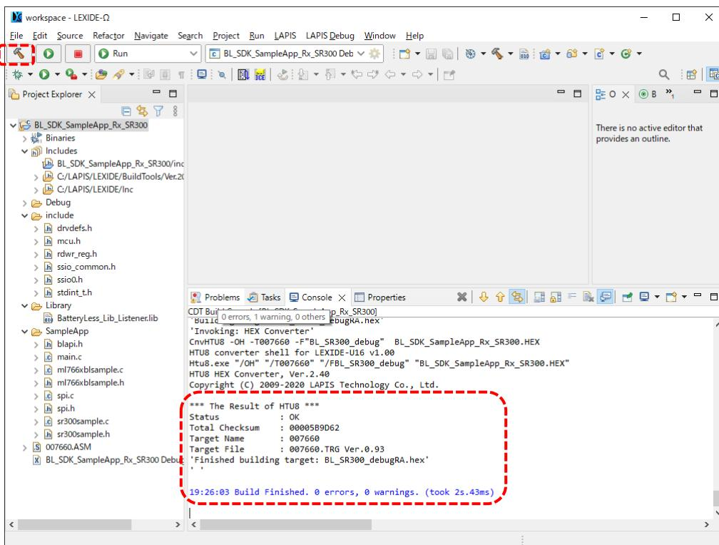
Step-6. Connect the EASE100V2 to the Rx board, download the above build results to the chip, and start debugging.
