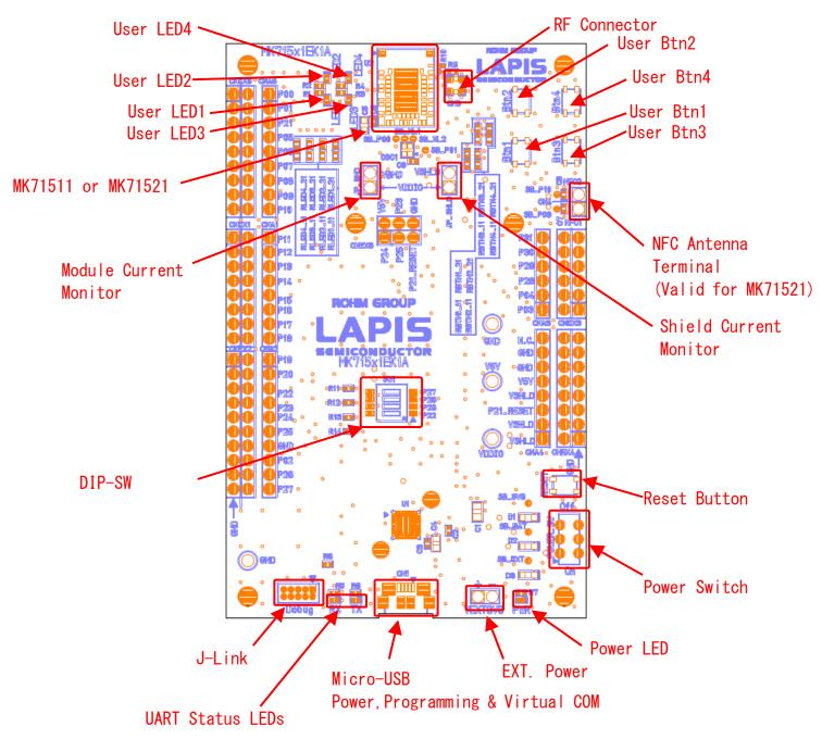
Fig. 2-1: Layout of MK715x1EK1A (Top View)
