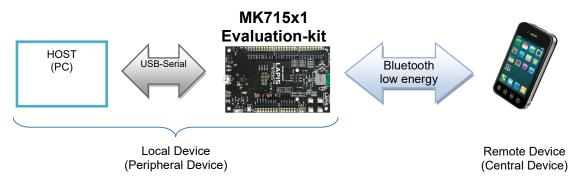
Fig. 3-1 : System configuration (when connecting to a smartphone, etc.)
