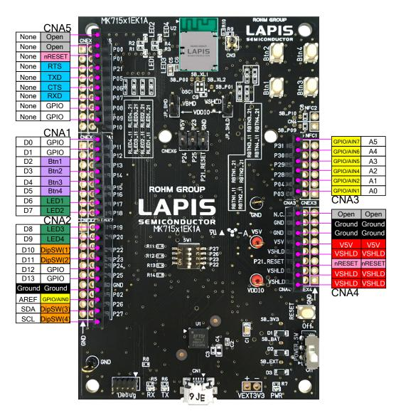
Fig. 2-12 : pin assignment table for External interface
