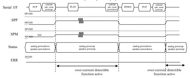
over-current detectible function for Speaker pins
