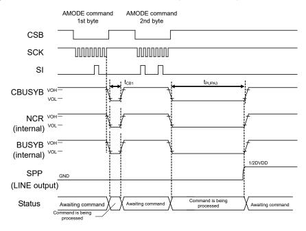
• When putting the speaker amplifier into the power down state Setting values: POP bit = "0", DAEN and SPEN bits = "1"  $\rightarrow$  "0"
