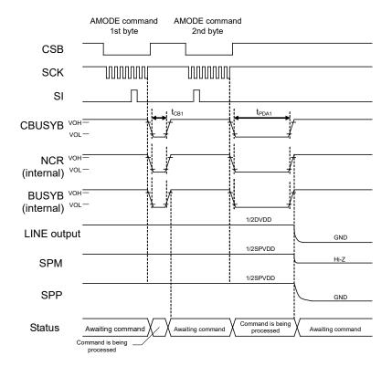
• When putting the line amplifier into the power down state (with pop noise suppression) Setting values: POP bit = "1", DAEN bit = "1"  $\rightarrow$  "0" (SPEN bit = "0")
