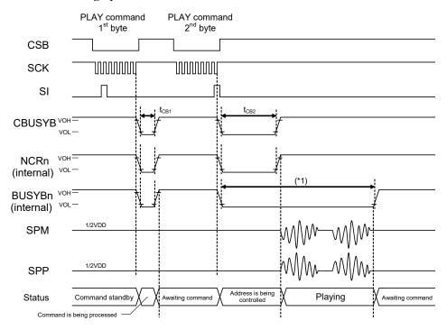
\*1: Length of the "L" interval of BUSYBn is =  $t_{CB2}$  + voice production time length.
