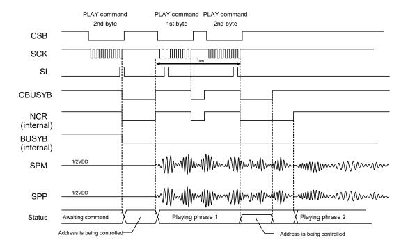
As shown in the diagram above, if performing continuous playback, input the PLAY command for the second phrase within  $10 \text{ ms (t_{cm})}$  after the NCR signal on the target channel goes "H". Please input the following PLAY command after checking that playback is completed by the RDSTAT command, when it is not continuous playback.
