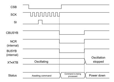
Oscillation stops after a lapse of command processing time after the PDWN command is input. The regulator stops operation after a lapse of command processing time after the PDWN command is input. At this time, the SPM output of the speaker amplifier goes into a Hi-Z state to prevent generation of pop noise.
