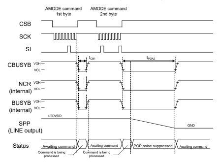
• When putting the line amplifier into the power down state (without pop noise suppression) Setting values: POP bit = "0", DAEN bit = "1"  $\rightarrow$  "0" (SPEN bit = "0")
