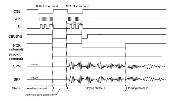
As shown in the diagram above, if performing continuous playback, input the START command for the second phrase within  $10 \text{ ms } (t_{cm})$  after the NCR signal on the target channel goes "H". Please input the following START command after checking that playback is completed by the RDSTAT command, when it is not continuous playback.
