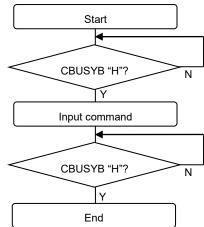
2-Byte Command Input Flow (applied to the AMODE, AVOL, FAD, FADR, PLAY, MUON, CVOL, and SAFE commands)
