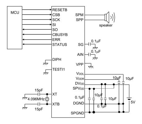
At using external speaker amplifier (line output)
