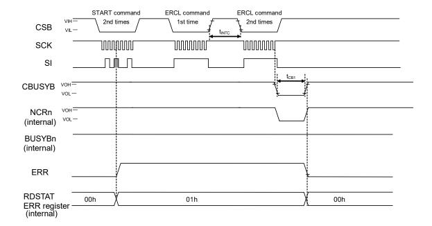
If a power supply voltage error occurs and then the power supply voltage is returned (when the SAFE command's BLD2-0 bits = 001h)
