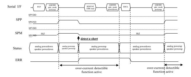
over-current detectible function Operation Flow (Example)
