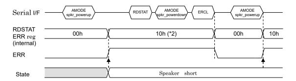
When ERCL is inputed before Error Clear Flow(\*1).
