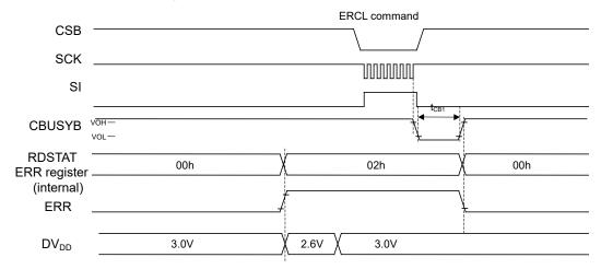
If a power supply voltage error occurs but the power supply voltage is not returned
