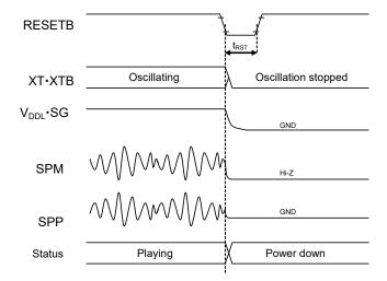
Note: The same timing applies in cases where the Reset signal is input during waiting for command.
