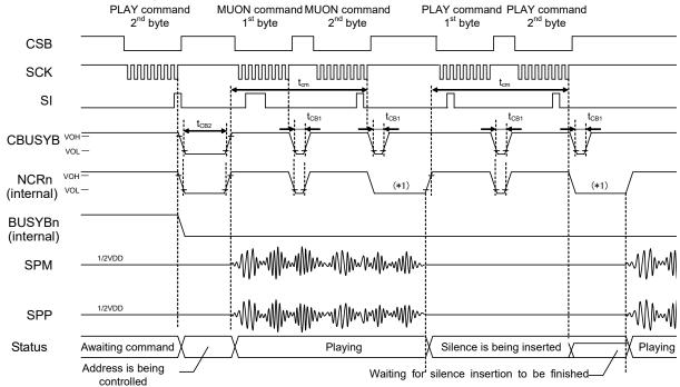
\*1: The "L" level period of the NCR pin during playback or silence insertion operation varies depending on the timing at which the MUON command is input.
