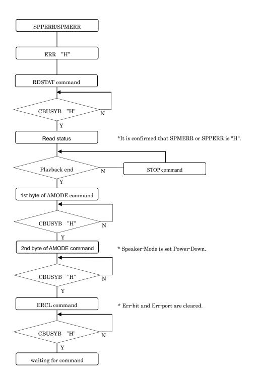
1-Byte Command input flow of two-time command input mode (applied to the PDWN, STOP, SLOOP, CLOOP, RDSTAT, OUTSTAT, and ERCL commands)
