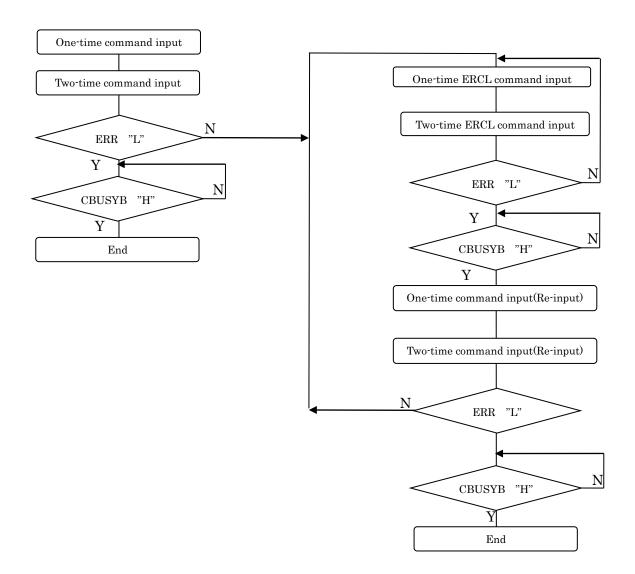
2-Byte Command input flow of two-time command input mode (applied to the AMODE, AVOL, FADR, PLAY, MUON, CVOL, and SAFE commands)
