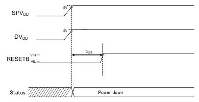
Oscillation is stopped after power-on. Be sure to set "L"level the RESETB pin before the first command input.
