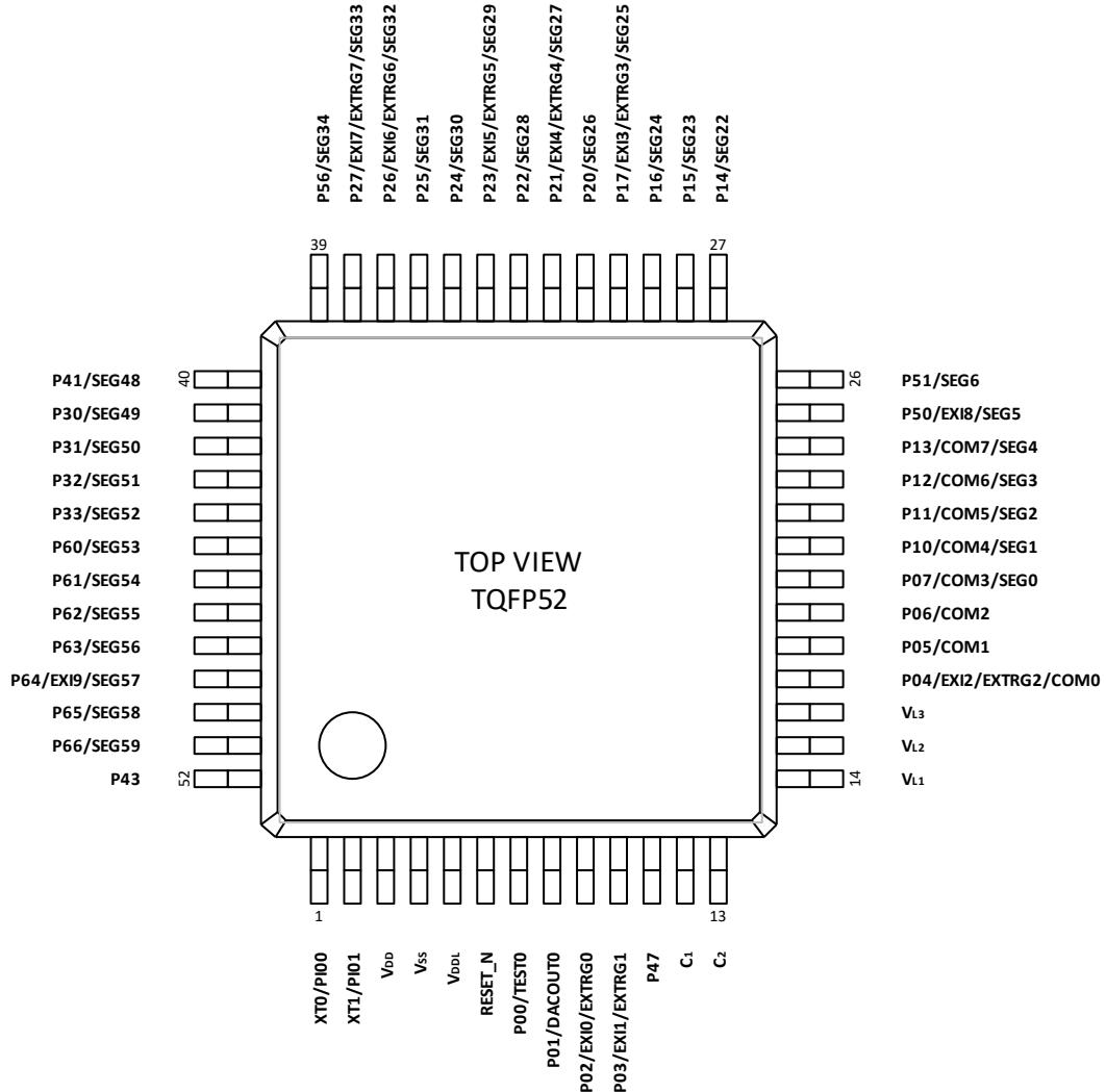
Figure 3 Pin Layout of 52pin TQFP52 Package
