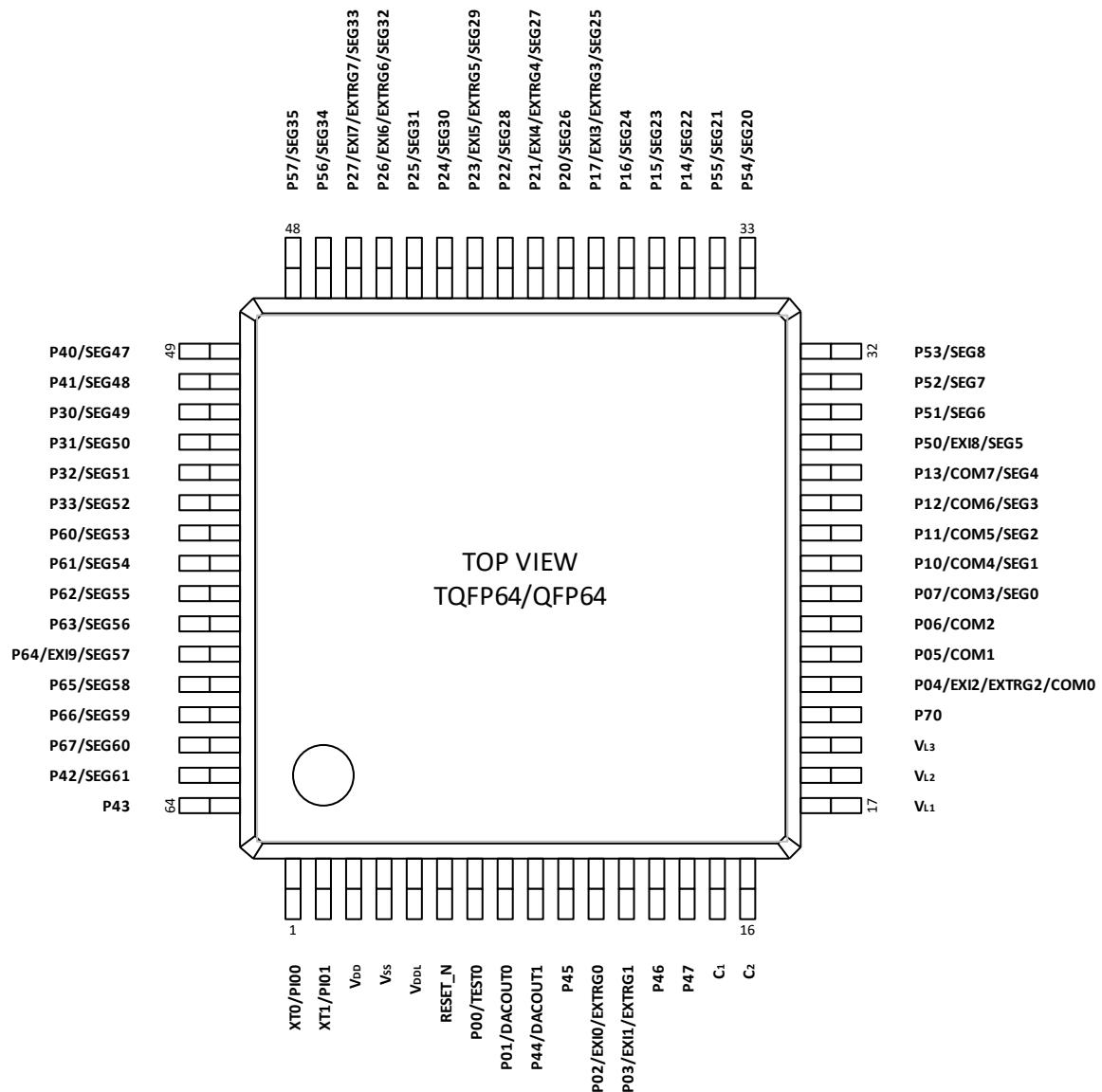
Figure 4 Pin Layout of 64pin TQFP/QFP Package
