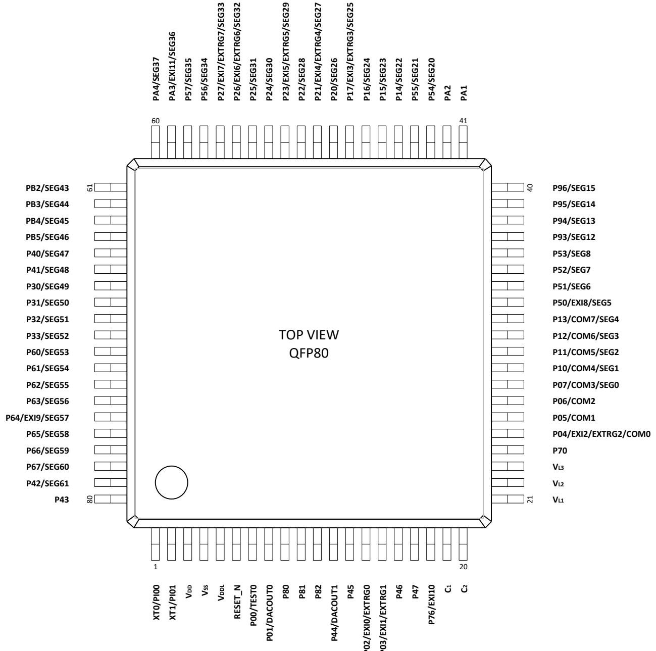
Figure 5 Pin Layout of 80pin QFP Package
