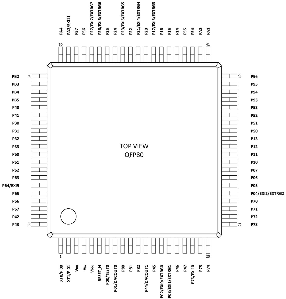
Figure 5 Pin Layout of 80pin QFP Package
