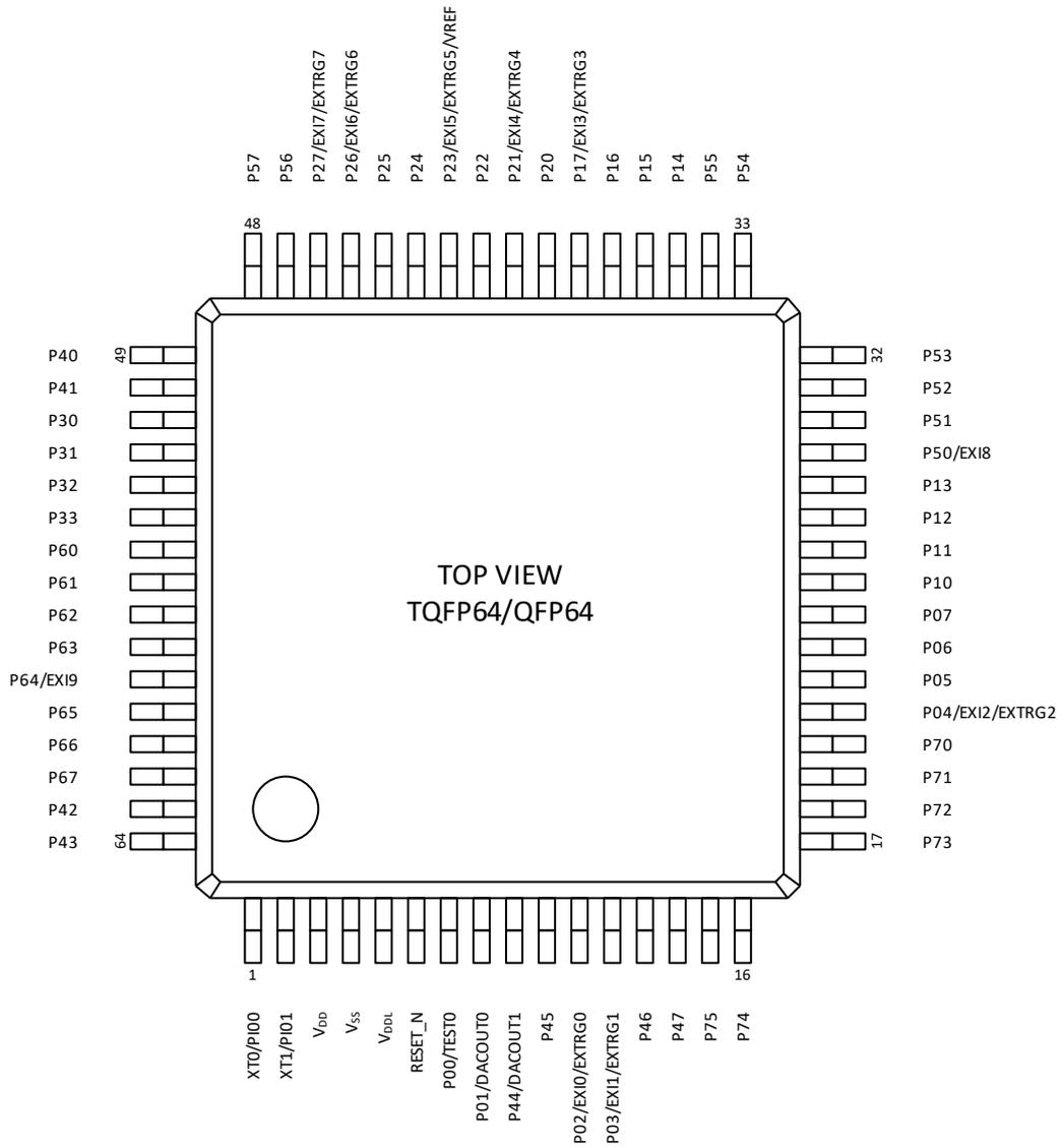
Figure 4 Pin Layout of 64pin TQFP/QFP Package
