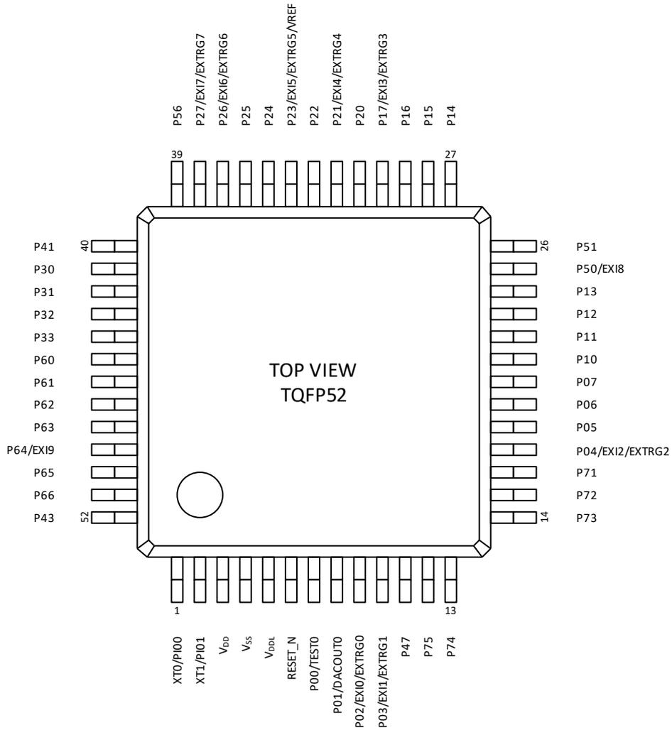
Figure 3 Pin Layout of 52pin TQFP52 Package
