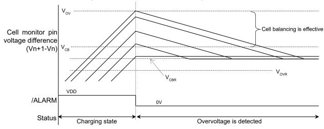
Cell balancing is executed at cells whose voltage is between over voltage detection threshold  $V_{\rm OV}$  and cell balancing detection threshold  $V_{\rm CB}$ .
