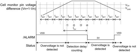
• In case if the overvoltage detection delay counting is not initialized
