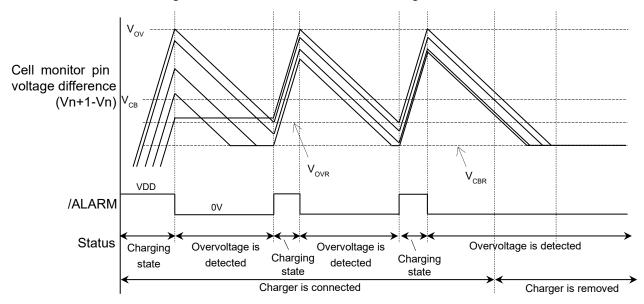
When the charger is connected, charging and discharging by cell balancing is repeated. When the charger is removed, the cell monitor voltage difference (Vn+1-Vn) will settle in cell balancing release threshold  $V_{CBR}$ .
