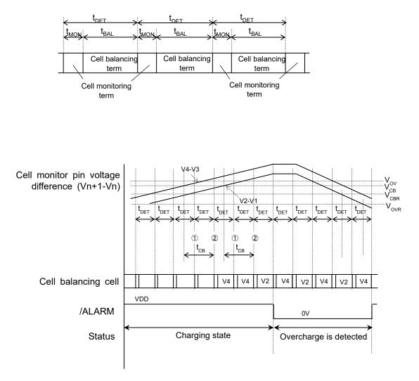
Cell balancing operation is shown below.
