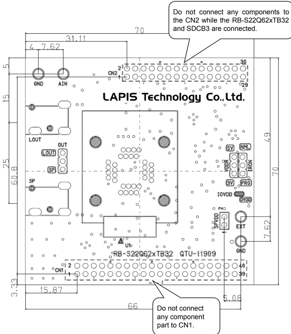
Figure 7 PCB layout
