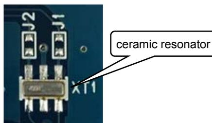
Figure 4 Ceramic resonator
