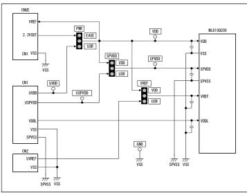
Figure 2 Jumper pin and Power circuit
