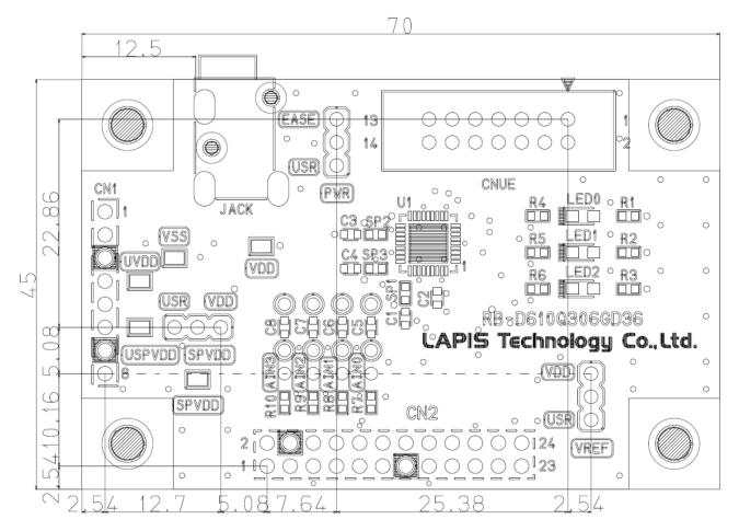
Figure 5 PCB layout
