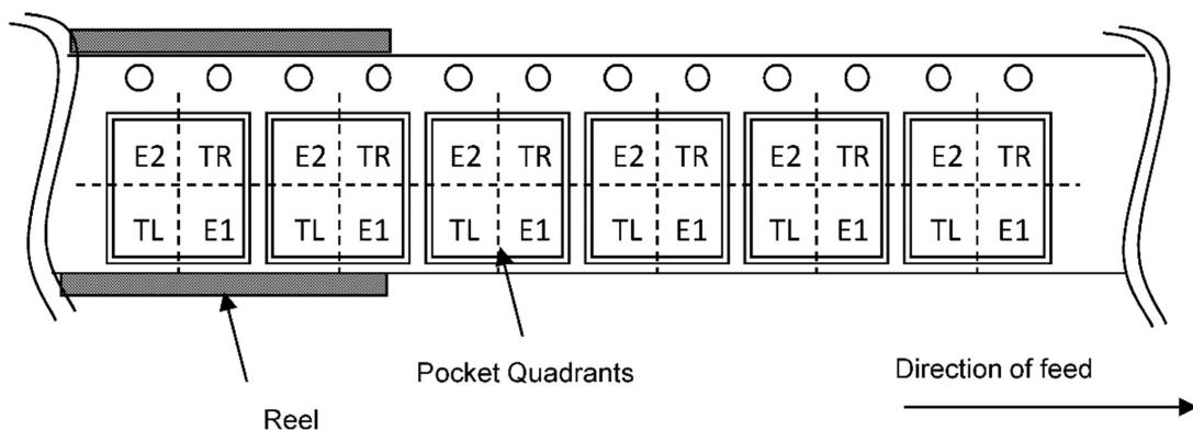
E2 : PIN1 is placed to the top left corner. TR : PIN1 is placed to the top right corner.
