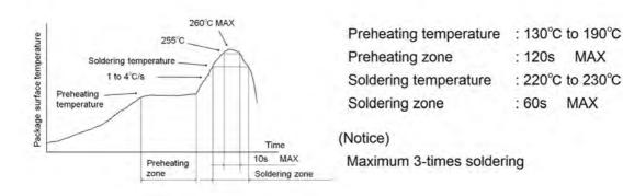
7.2. About mounting with Sn-Pb solder paste
