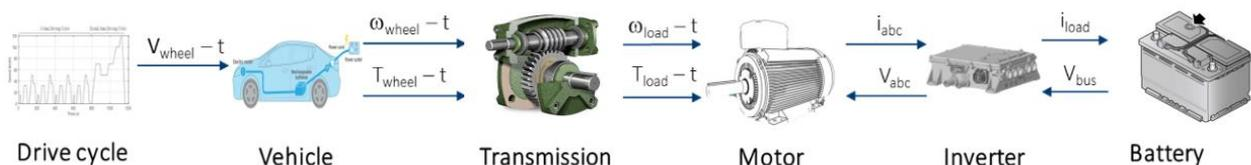
Fig. 10: Concept diagram of endurance mileage evaluation for electrical vehicle
