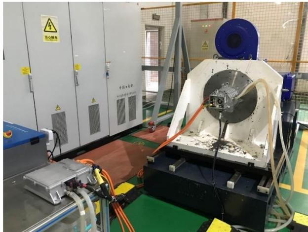
Fig. 4: Efficiency test of SiC motor controller
