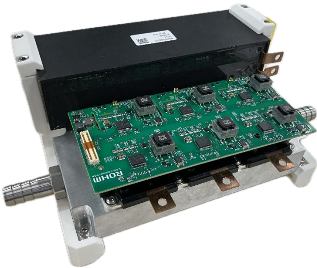
Figure 3. 3 phase Inverter EVK (assembled with KIT)
