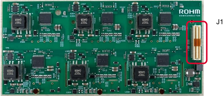
Figure 8. J1 location on the GD Board
