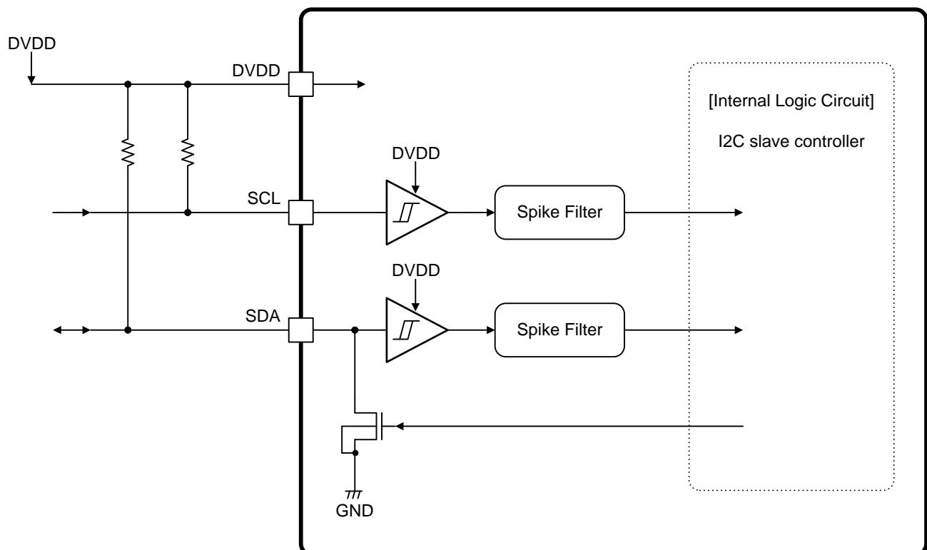
Figure 4-1. I<sup>2</sup>C (Slave) Block Diagram
