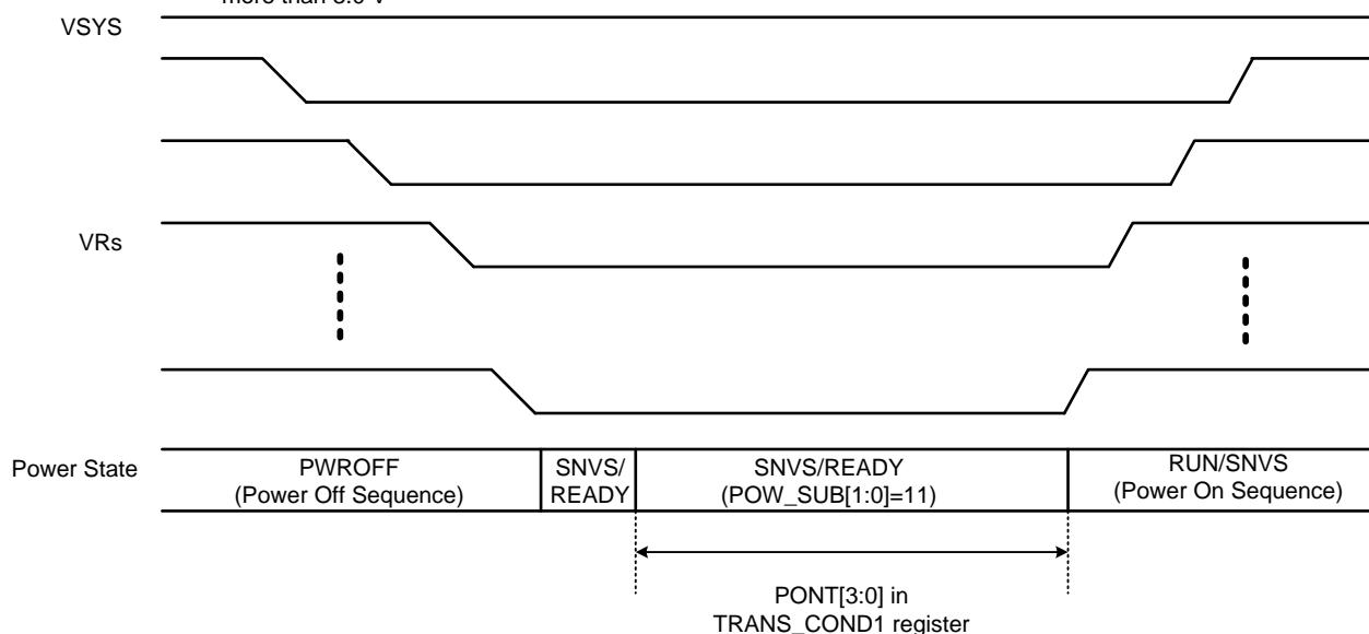
Figure 3-19. Cold Reset Duration Time set by PONT[3:0]
