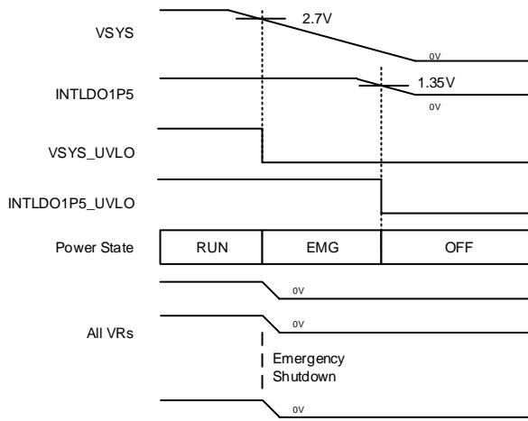
Figure 3-15. EMG to OFF Power State Transition
