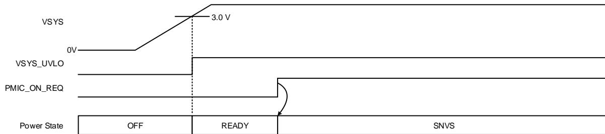
**Figure 3-5. PMIC\_ON\_REQ Condition for moving to SNVS**
