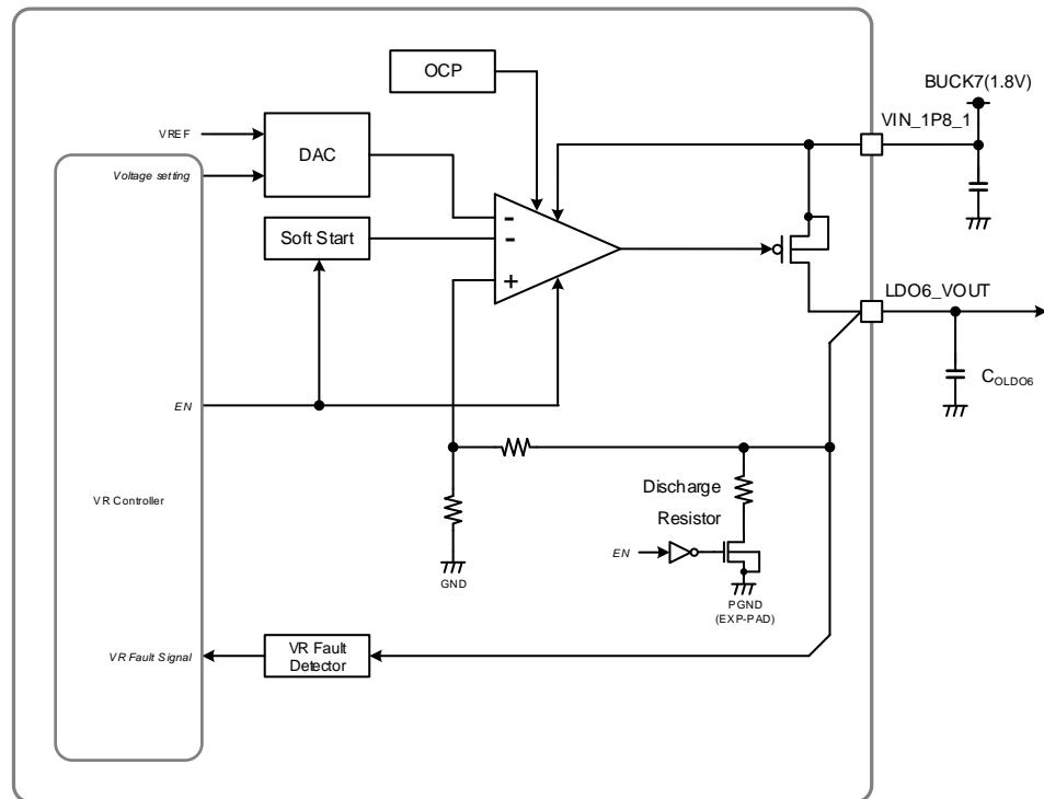
Figure 5-14. LDO6 Block Diagram
