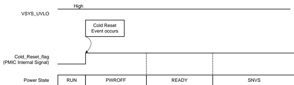
**Figure 3-8. Cold Reset Condition for moving to SNVS**
