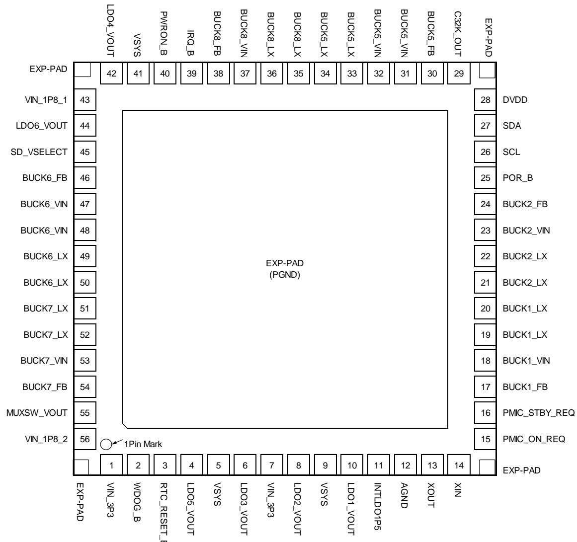
Figure 1-3. Pin Configuration (TOP VIEW)
