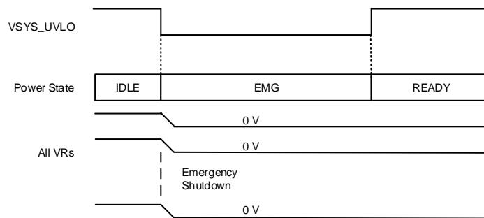
**Figure 3-16. EMG to READY Power State Transition (VSYS\_UVLO)**
