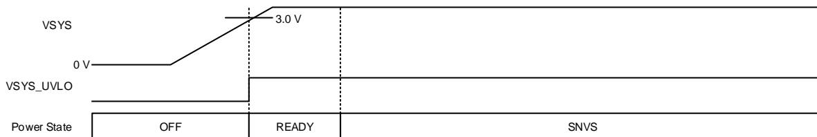
**Figure 3-4. VSYS Condition for moving to SNVS**
