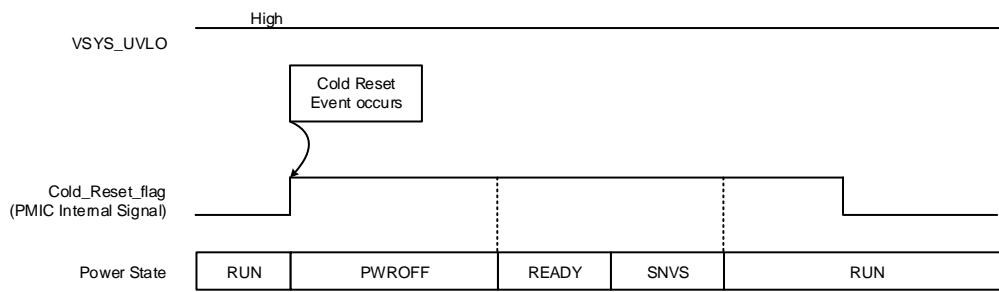
**Figure 3-13. Cold Reset Condition for moving to RUN**
