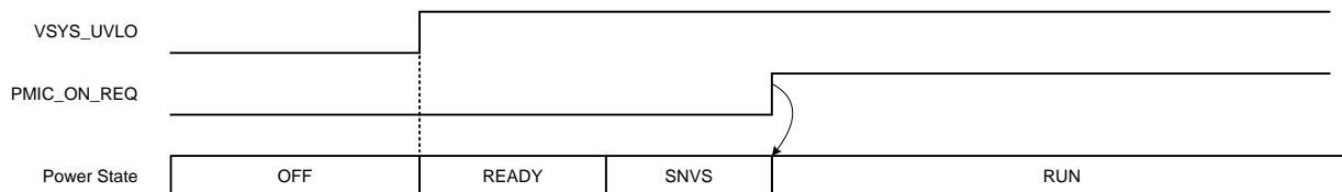
**Figure 3-10. PMIC\_ON\_REQ Condition for moving to RUN**
