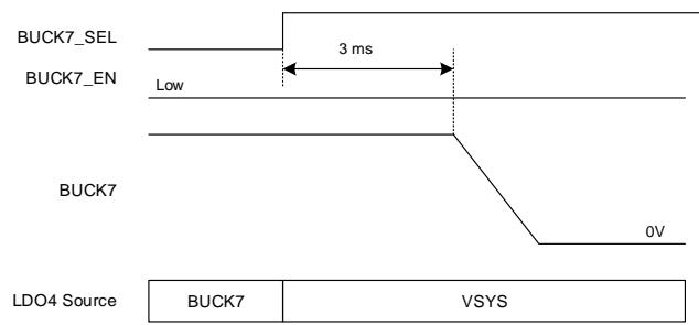
**Figure 5-12. LDO4 Voltage Source Switching**
