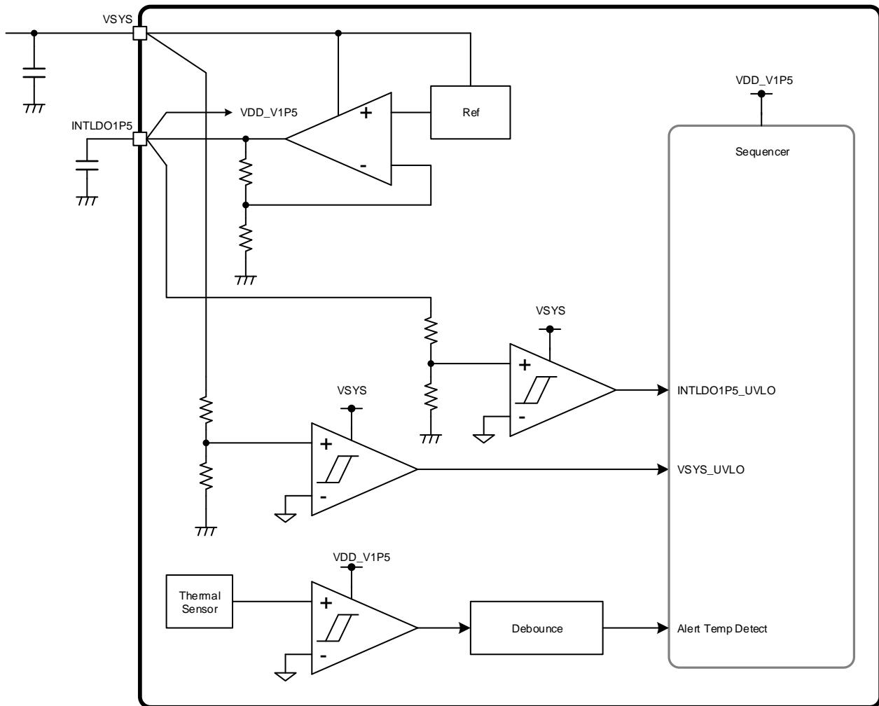
Figure 2-1. Power Reference and Detectors Block Diagram
