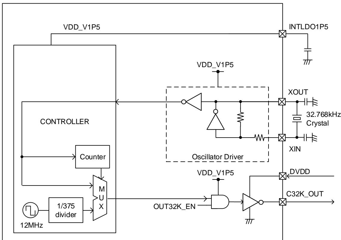
Figure 6-1. 32.768 kHz Crystal Oscillator Driver Block Diagram
