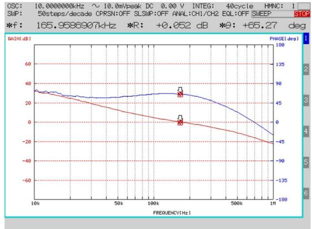
Figure 47. Frequency Characteristics ( $I_{OUT} = 0.5\text{ A}$ )
