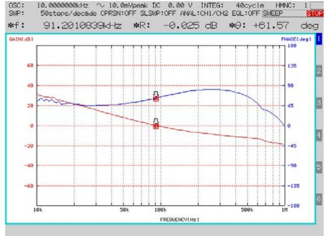
Figure 52. Frequency Characteristics ( $I_{OUT} = 0.5\text{ A}$ )
