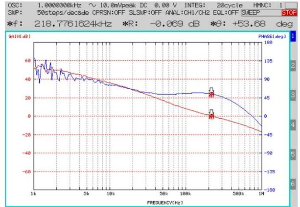
Figure 37. Frequency Characteristics ( $I_{OUT} = 0.5\text{ A}$ )
