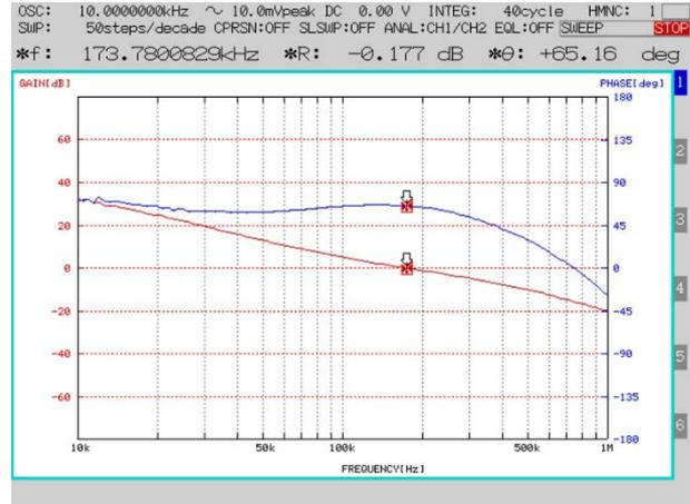
Figure 42. Frequency Characteristics ( $I_{OUT} = 0.5\text{ A}$ )
