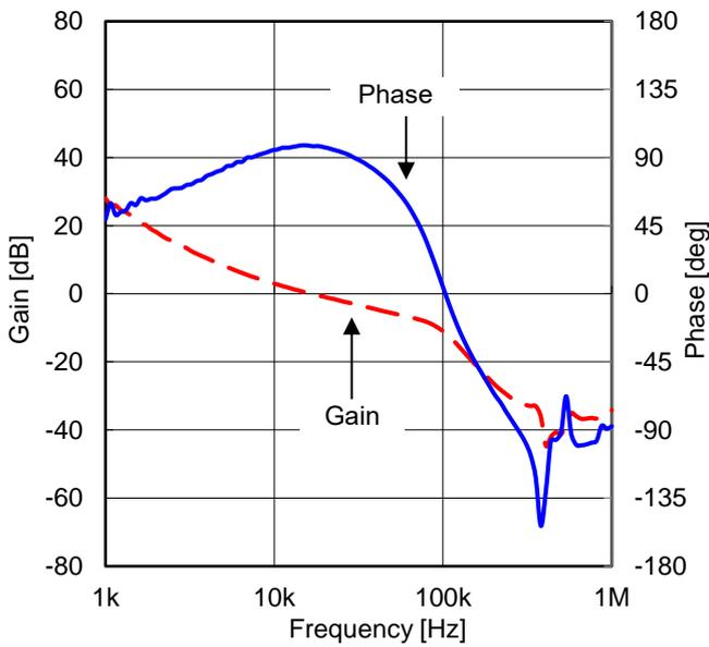
Figure 78. Frequency Characteristic (VIN = 12 V, IOUT = 1.0 A)
