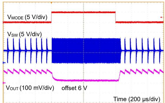
Figure 53. MODE ON/OFF Response (VIN = 12 V, IOUT = 50 mA)
