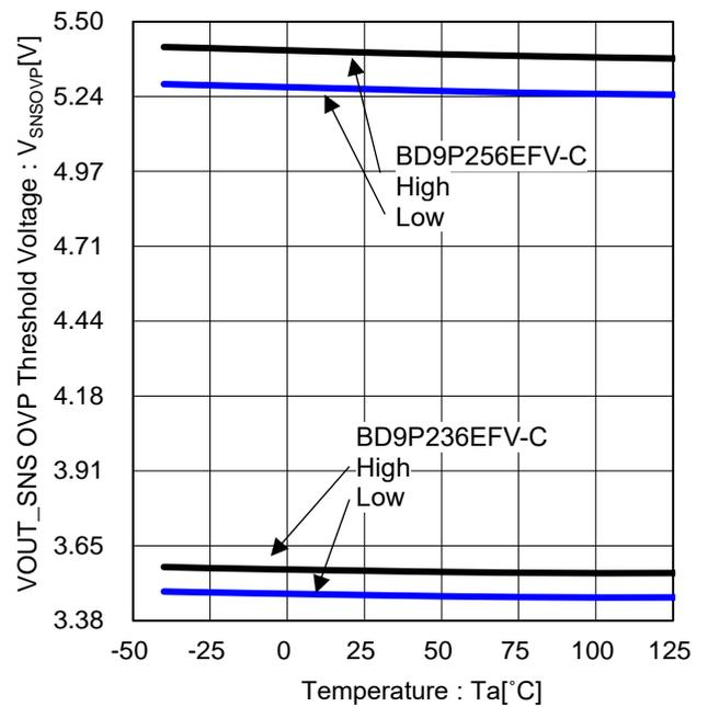
Figure 28. VOUT\_SNS OVP Threshold Voltage vs Temperature (BD9P236EFV-C/BD9P256EFV-C)
