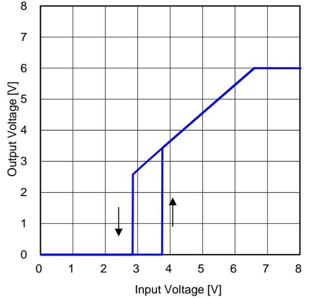
Figure 59. Output Voltage vs Input Voltage 2
