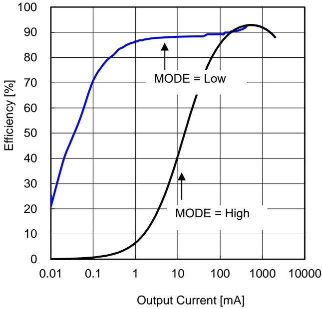
Figure 63. Efficiency vs Output Current (VIN = 12 V)
