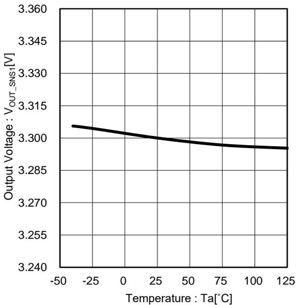
Figure 11. Output Voltage vs Temperature (BD9P236EFV-C)
