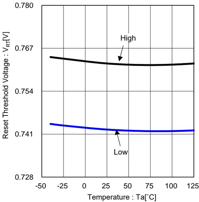
Figure 23. Reset Threshold Voltage vs Temperature (BD9P206EFV-C)
