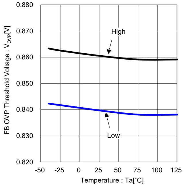
Figure 26. FB OVP Threshold Voltage vs Temperature (BD9P206EFV-C)
