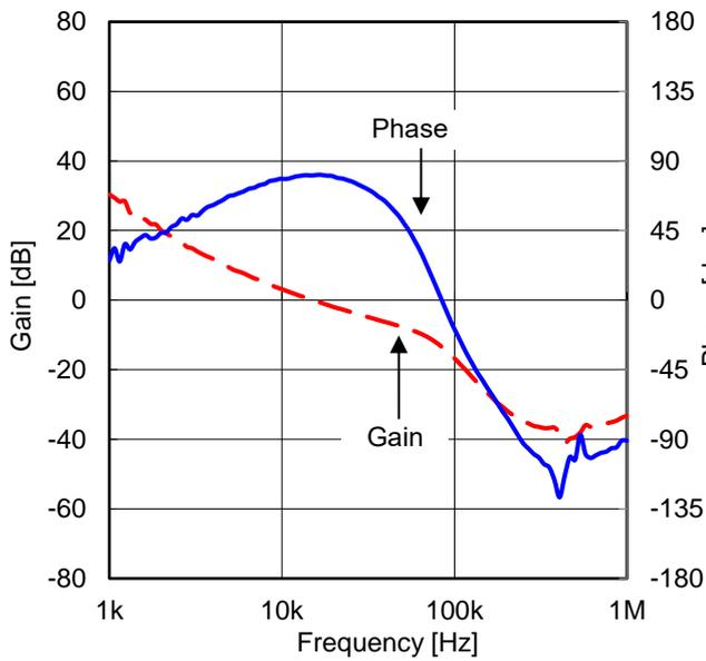
Figure 52. Frequency Characteristic (VIN = 12 V, IOUT = 1.0 A)
