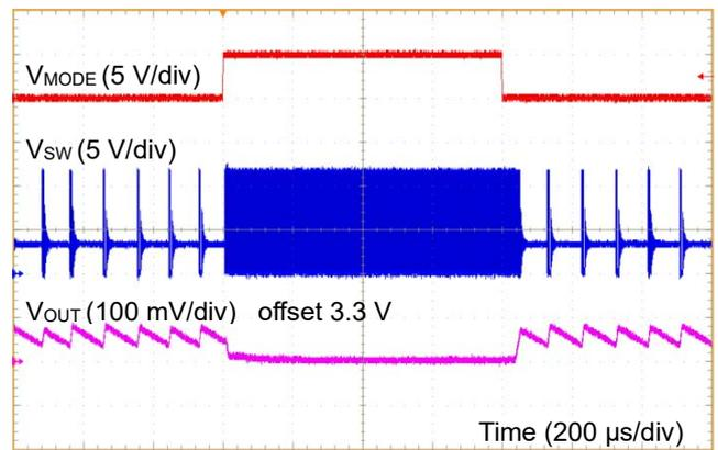
Figure 66. MODE ON/OFF Response (VIN = 12 V, IOUT = 50 mA)
