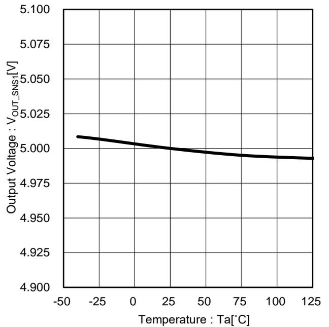
Figure 12. Output Voltage vs Temperature (BD9P256EFV-C)
