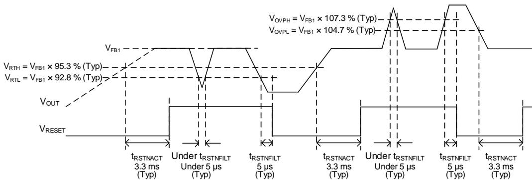
Figure 34. Reset Timing Chart (BD9P206EFV-C)
