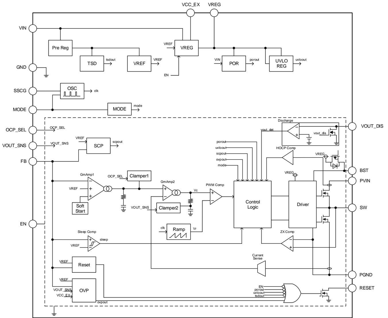
Figure 7. Block Diagram (BD9P206EFV-C)
