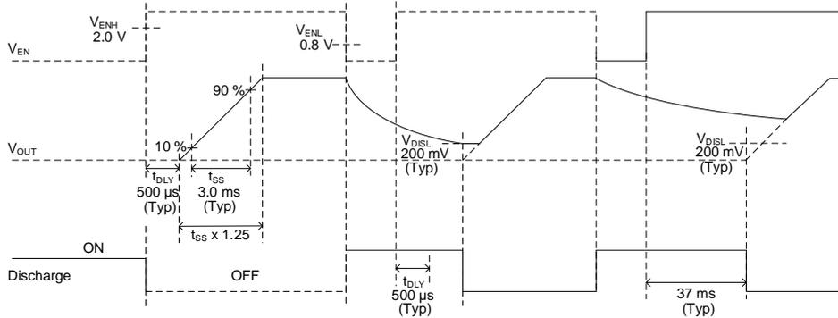
Figure 33. Enable ON/OFF Timing Chart
