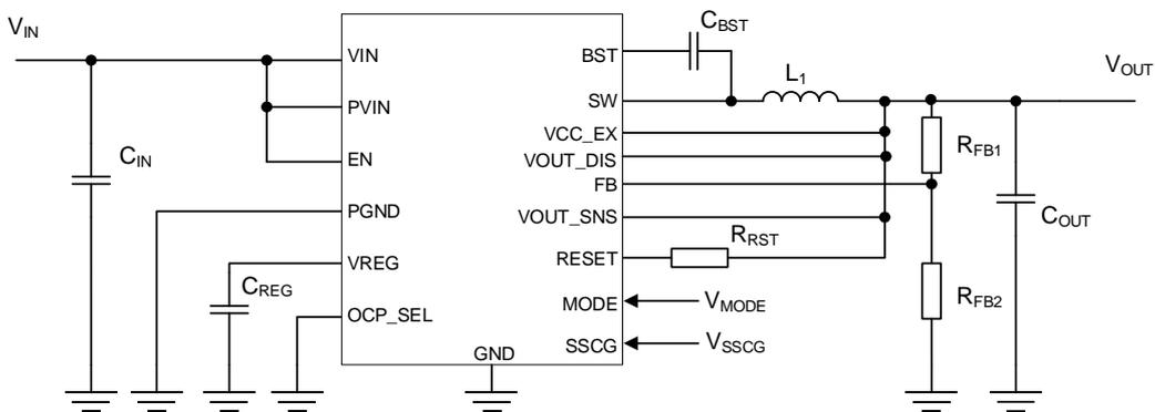
Figure 3. Application Circuit with Discharge Function (BD9P206EFV-C)
