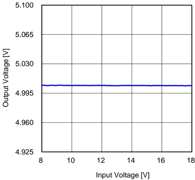
Figure 86. Line Regulation (I<sub>OUT</sub> = 2 A)
