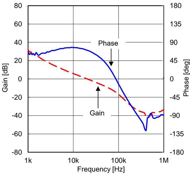
Figure 65. Frequency Characteristic (VIN = 12 V, IOUT = 1.0 A)
