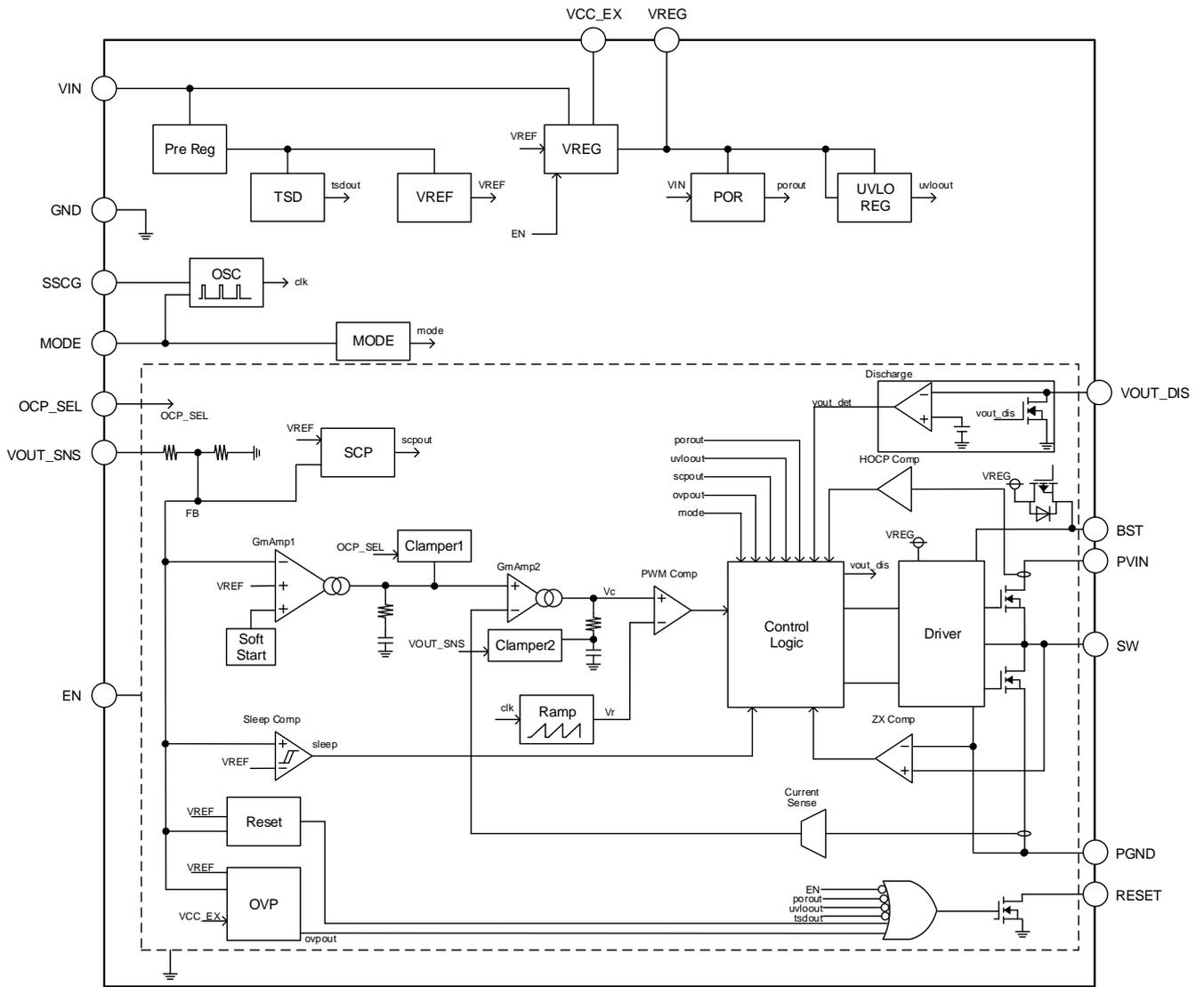
Figure 8. Block Diagram (BD9P236EFV-C, BD9P256EFV-C)
