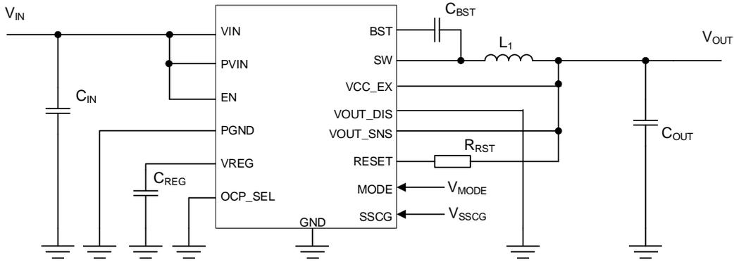
Figure 2. Application Circuit without Discharge Function (BD9P236EFV-C, BD9P256EFV-C)
