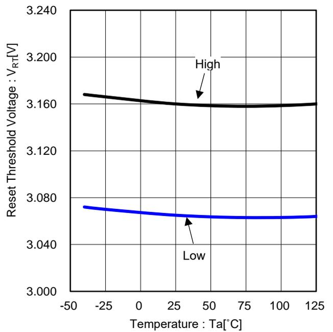
Figure 24. Reset Threshold Voltage vs Temperature (BD9P236EFV-C)
