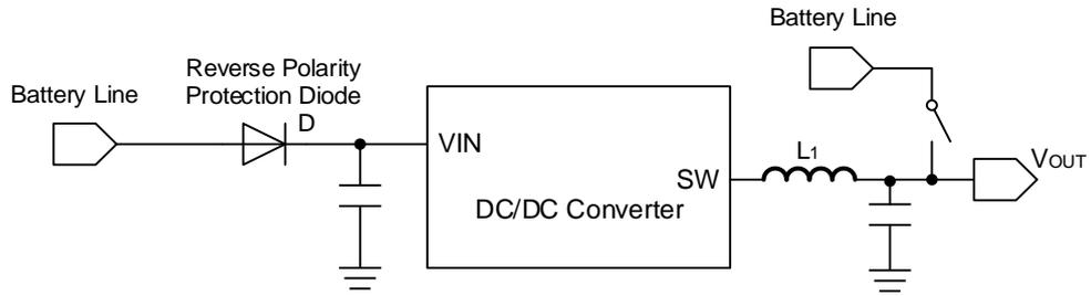
Figure 46. VOUT shorted to Battery Line
