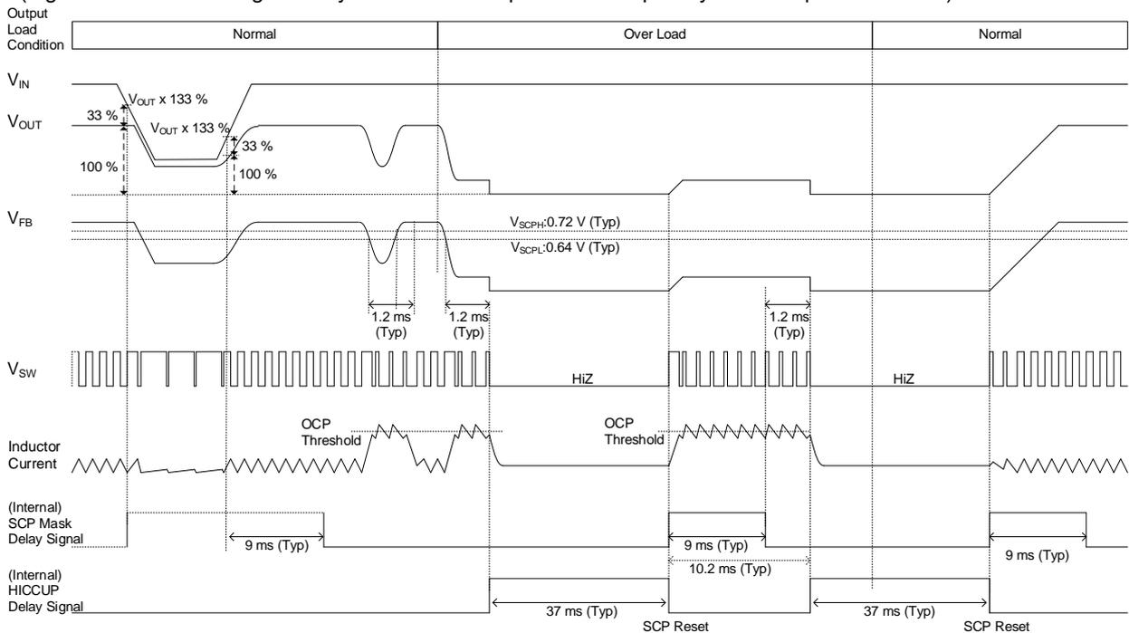
Figure 41. Short Circuit Protection (SCP) Timing Chart (BD9P206EFV-C)
