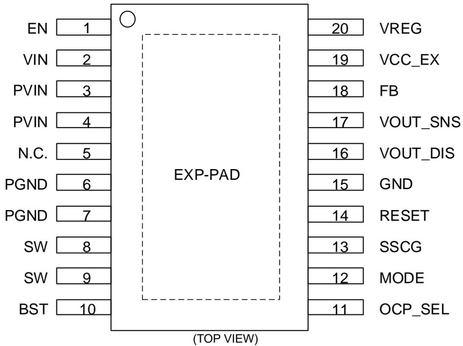
Figure 6. Pin Configuration (BD9P206EFV-C)
