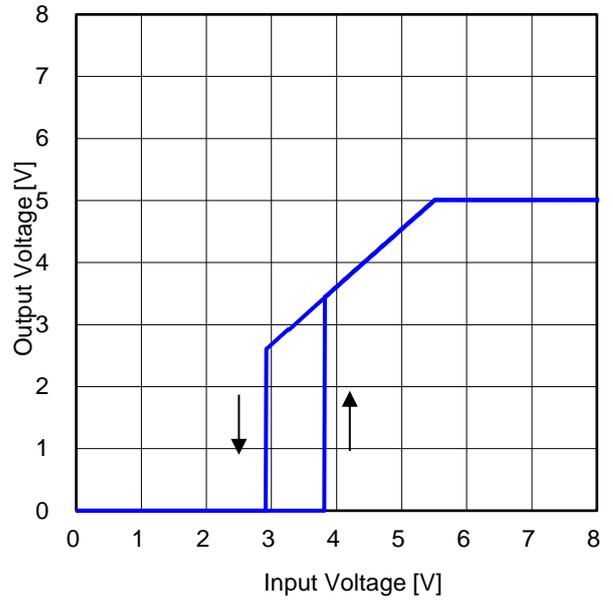
Figure 85. Output Voltage vs Input Voltage 2 (R<sub>LOAD</sub> = 2.5 Ω)
