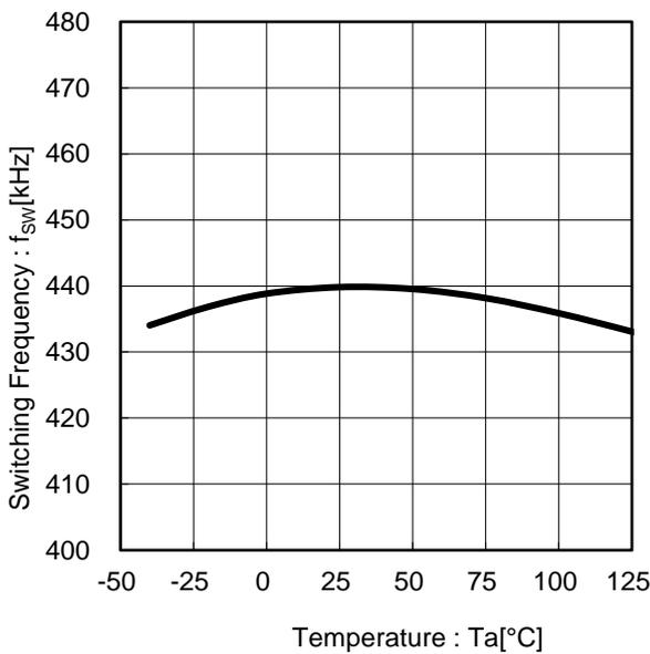
Figure 19. Switching Frequency vs Temperature
