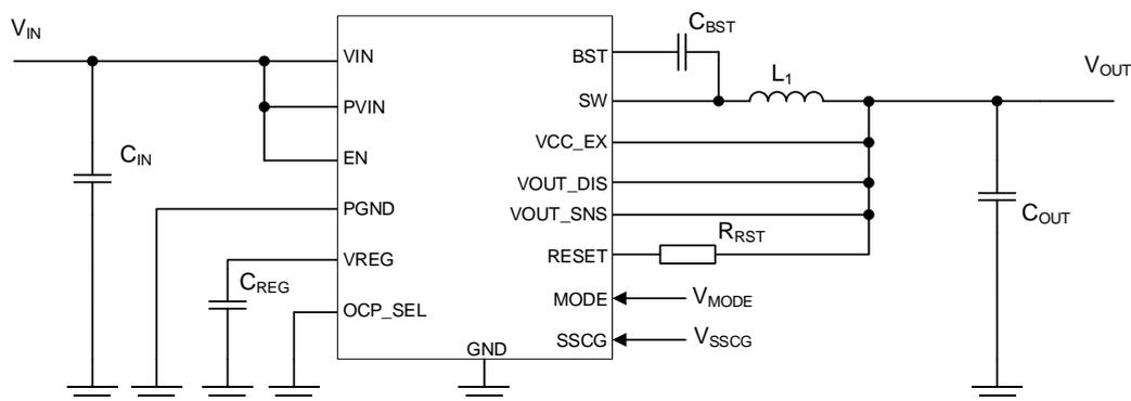
Figure 1. Application Circuit with Discharge Function (BD9P236EFV-C, BD9P256EFV-C)
