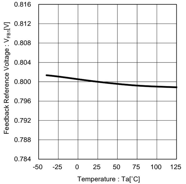
Figure 10. Feedback Reference Voltage vs Temperature (BD9P206EFV-C)
