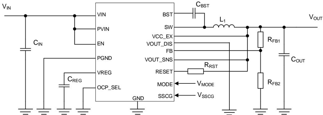
Figure 4. Application Circuit without Discharge Function (BD9P206EFV-C)
