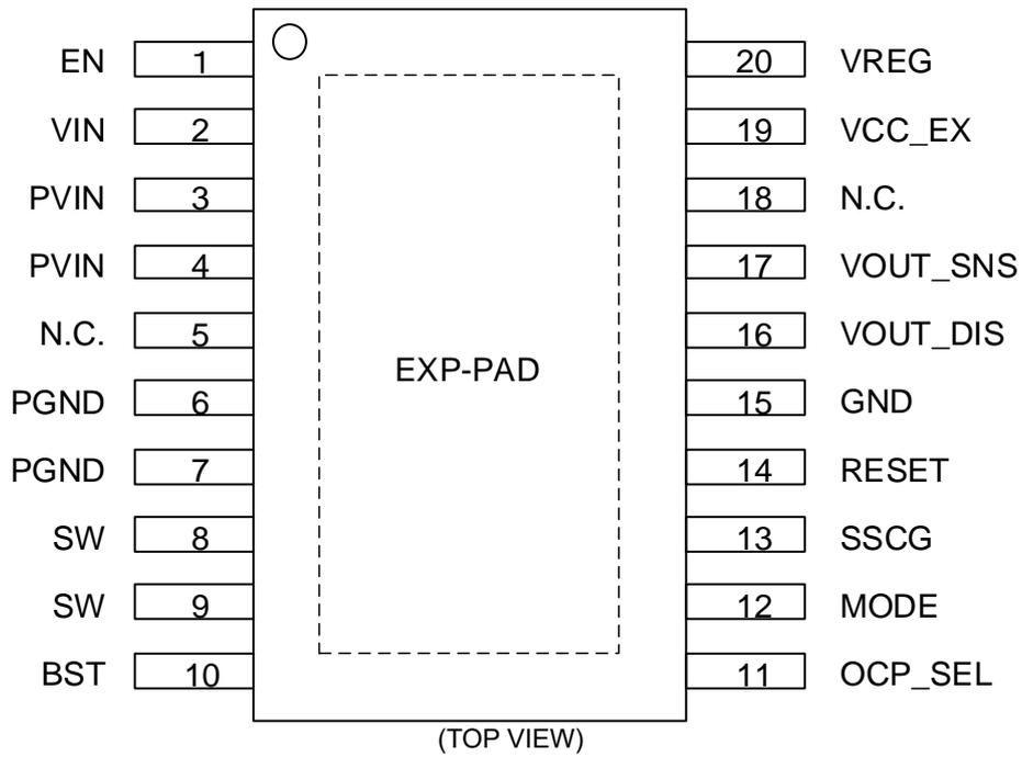
Figure 5. Pin Configuration (BD9P236EFV-C, BD9P256EFV-C)
