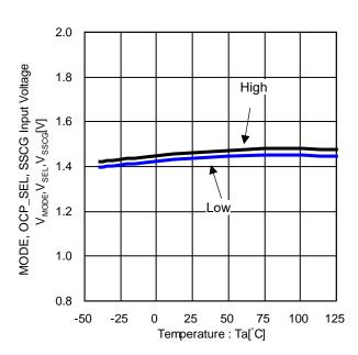
Figure 11. MODE, OCP\_SEL, SSCG Input Voltage vs Temperature
