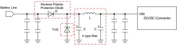
Figure 66. Automotive Power Supply Line Circuit
