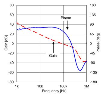
Figure 43. Frequency Characteristic  $(V_{IN} = 12 V, I_{OUT} = 1.0 A)$
