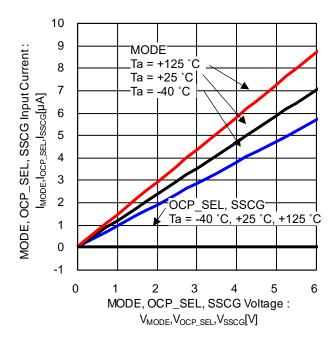
Figure 12. MODE, OCP\_SEL, SSCG Input Current vs MODE, OCP\_SEL, SSCG Voltage
