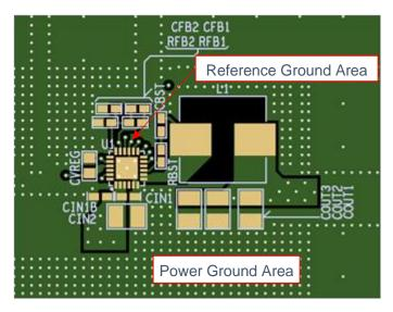
Figure 68. Recommended Board Layout Example
