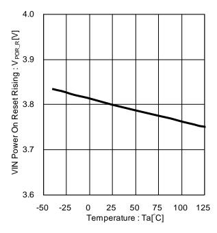
Figure 7. VIN Power On Reset Rising vs Temperature
