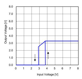
Figure 50. Output Voltage vs Input Voltage 2  $(R_{LOAD} = 1.65 \Omega)$
