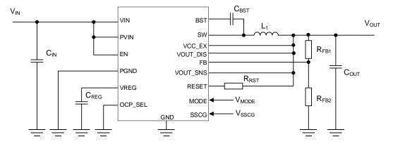
Figure 1. Application Circuit with Discharge Function
