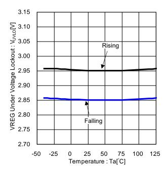
Figure 8. VREG Under Voltage Lockout vs Temperature
