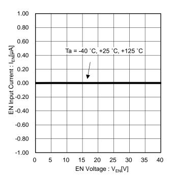
Figure 10. EN Input Current vs EN Voltage
