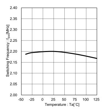
Figure 13. Switching Frequency vs Temperature
