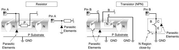
Figure 71. Example of Monolithic IC Structure
