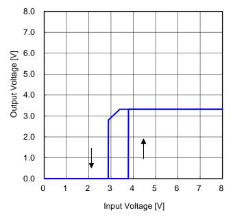
Figure 49. Output Voltage vs Input Voltage 1  $(R_{LOAD} = 165 \Omega)$
