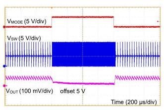
Figure 57. MODE ON/OFF Response ( $V_{IN} = 12 \text{ V}, I_{OUT} = 50 \text{ mA}$ )
