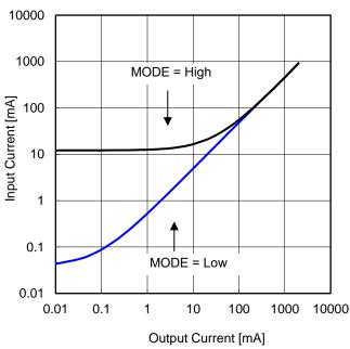
Figure 55. Input Current vs Output Current (V<sub>IN</sub> = 12 V)
