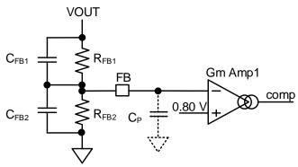
Figure 39. Setting for Output Setting Resistor
