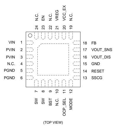
Figure 3. Pin Configuration
