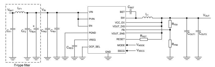
Figure 53. Reference Circuit 2
