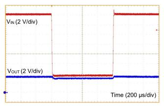
Figure 47. Line Response 1  $(V_{IN} = 16 \text{ V to 8 V, } I_{OUT} = 2 \text{ A})$
