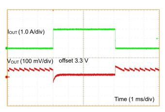
Figure 45. Load Response 1 ( $V_{IN}$  = 12 V,  $V_{MODE}$  = 5 V,  $I_{OUT}$  = 0 A to 2 A)
