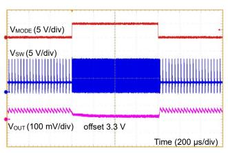
Figure 44. MODE ON/OFF Response  $(V_{IN} = 12 \text{ V}, I_{OUT} = 50 \text{ mA})$
