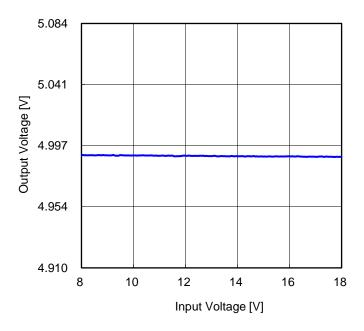
Figure 64. Line Regulation (I<sub>OUT</sub> = 2 A)
