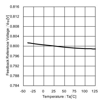
Figure 6. Feedback Reference Voltage vs Temperature
