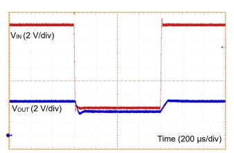
Figure 60. Line Response 1 ( $V_{IN}$  = 16 V to 8 V,  $I_{OUT}$  = 2 A)
