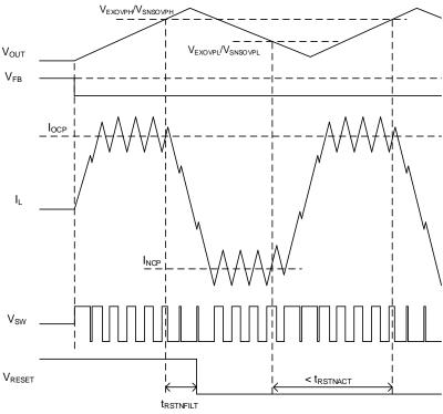
Figure 36. VCC\_EX/VOUT\_SNS OVP Timing Chart
