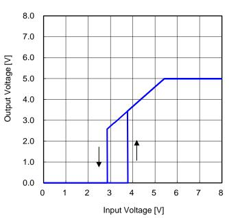
Figure 63. Output Voltage vs Input Voltage 2  $(R_{LOAD} = 2.5 \Omega)$
