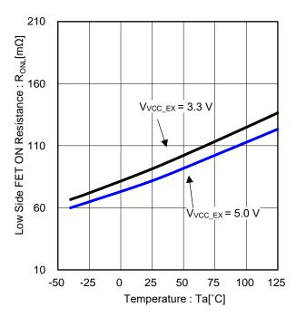
Figure 16. Low Side FET ON Resistance vs Temperature
