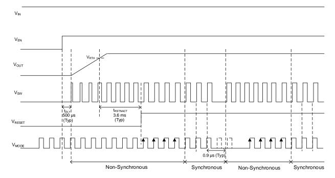
Figure 26. External Synchronization Function
