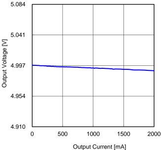
Figure 65. Load Regulation (V<sub>IN</sub> = 12 V)
