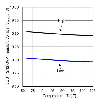
Figure 19. VOUT\_SNS OVP Threshold Voltage vs Temperature
