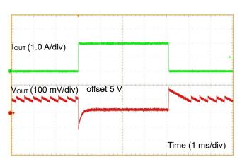
Figure 58. Load Response 1 ( $V_{IN}$  = 12 V,  $V_{MODE}$  = 5 V,  $I_{OUT}$  = 0 A to 2 A)
