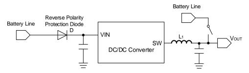
Figure 37. VOUT shorted to Battery Line
