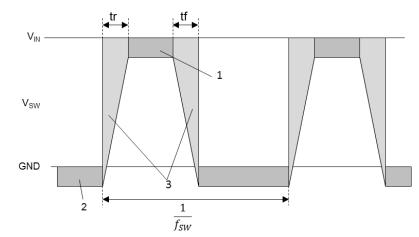
Figure 70. SW Waveform
