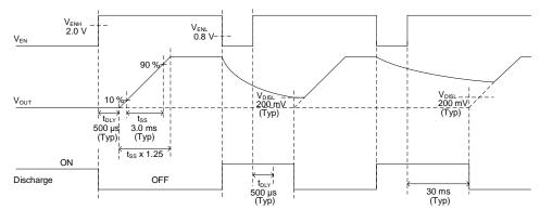
Figure 24. Enable ON/OFF Timing Chart
