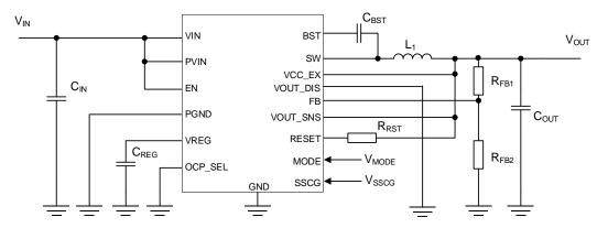
Figure 2. Application Circuit without Discharge Function
