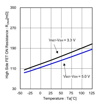
Figure 15. High Side FET ON Resistance vs Temperature
