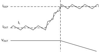
Figure 31. Over Current Protection
