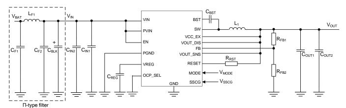
Figure 40. Reference Circuit 1
