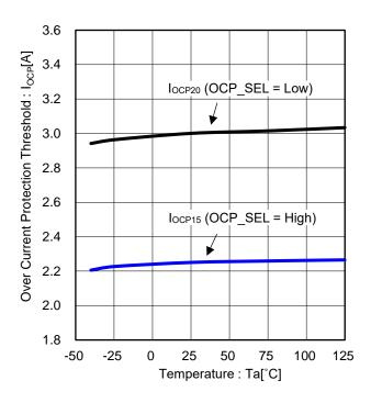
Figure 14. Over Current Protection Threshold vs Temperature
