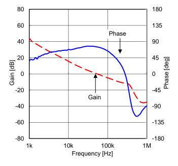
Figure 56. Frequency Characteristic ( $V_{IN}$  = 12 V,  $I_{OUT}$  = 1.0 A)
