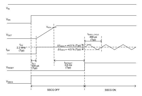
Figure 28. Spread Spectrum Function
