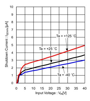
Figure 5. Shutdown Current vs Input Voltage
