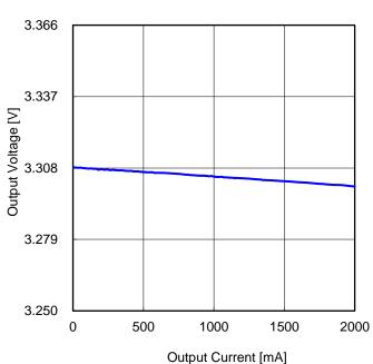
Figure 52. Load Regulation (V<sub>IN</sub> = 12 V)
