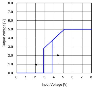
Figure 62. Output Voltage vs Input Voltage 1  $(R_{LOAD} = 250 \Omega)$
