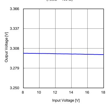
Figure 51. Line Regulation (I<sub>OUT</sub> = 2 A)
