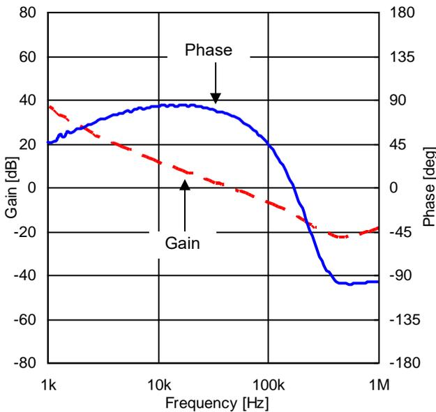
Figure 52. Frequency Characteristic (VIN = 12 V, IOUT = 0.5 A)
