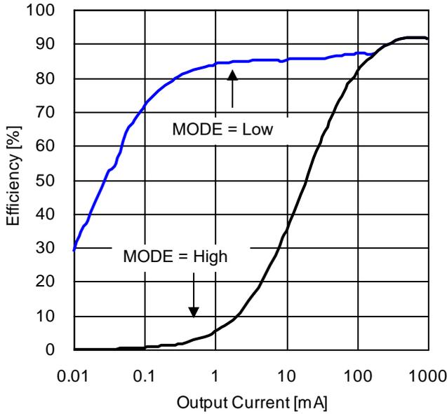
Figure 76. Efficiency vs Output Current (VIN = 12 V)
