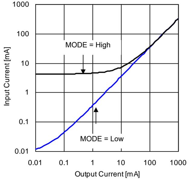
Figure 64. Input Current vs Output Current (VIN = 12 V)
