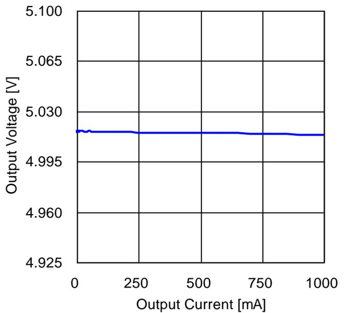
Figure 87. Load Regulation ( $V_{IN} = 12\ \text{V}$ )
