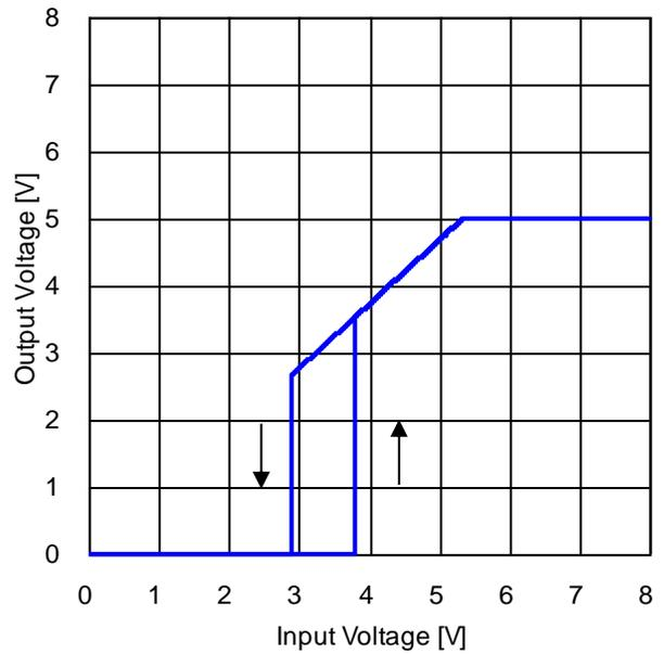
Figure 85. Output Voltage vs Input Voltage 2 ( $R_{LOAD} = 5\ \Omega$ )
