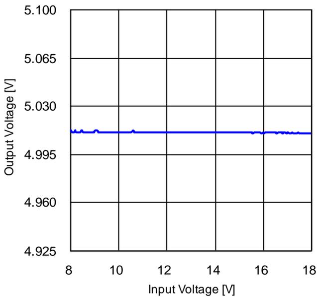
Figure 86. Line Regulation ( $I_{OUT} = 1\ \text{A}$ )
