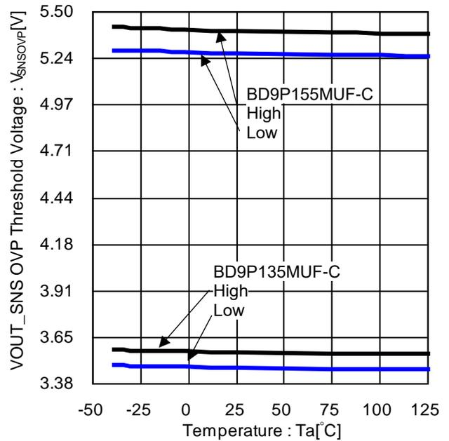
Figure 28. VOUT\_SNS OVP Threshold Voltage vs Temperature (BD9P135MUF-C/BD9P155MUF-C)
