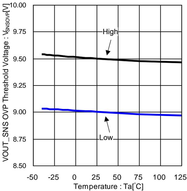
Figure 27. VOUT\_SNS OVP Threshold Voltage vs Temperature (BD9P105MUF-C)
