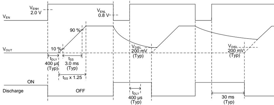
Figure 33. Enable ON/OFF Timing Chart
