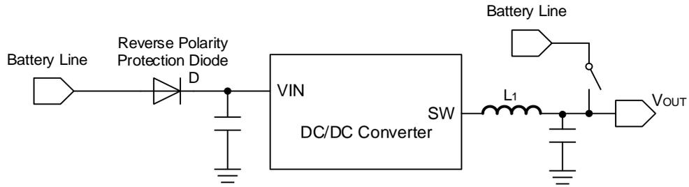
Figure 46. VOUT Shorted to Battery Line
