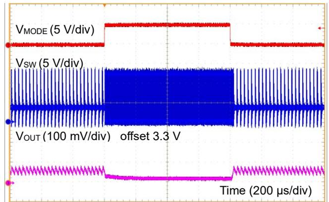
Figure 66. MODE ON/OFF Response (VIN = 12 V, IOUT = 50 mA)
