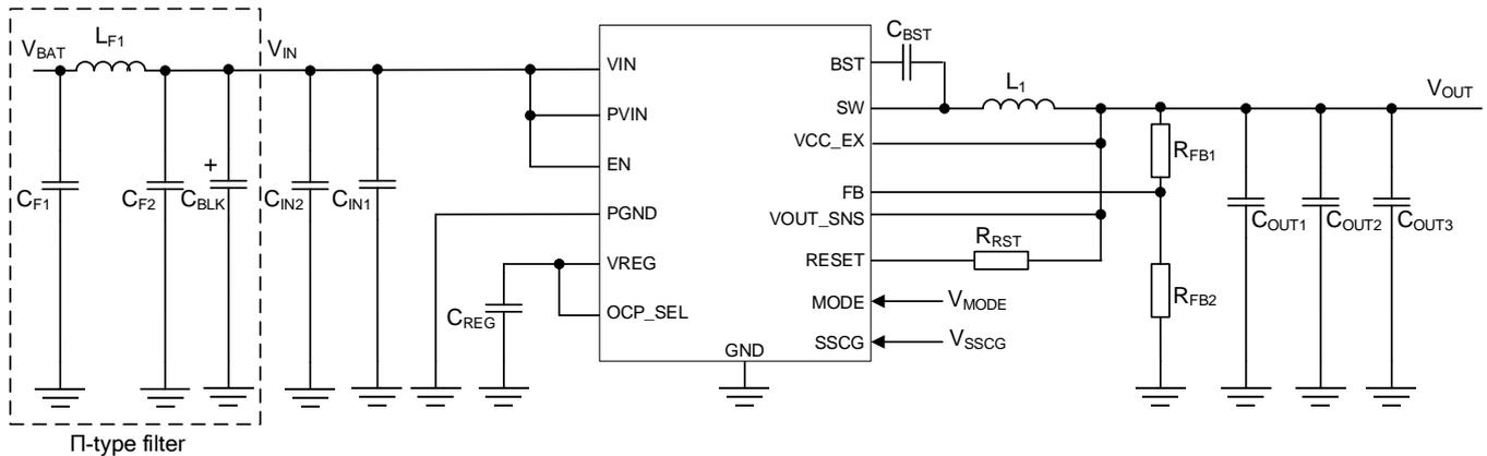
Figure 49. Reference Circuit 1
