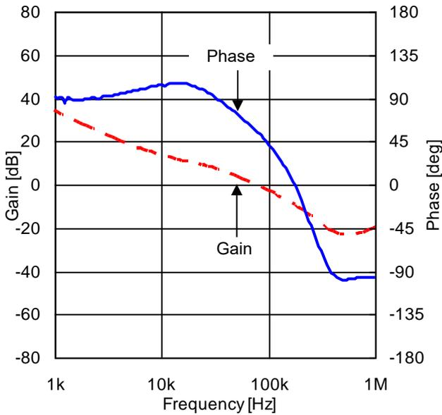
Figure 65. Frequency Characteristic (VIN = 12 V, IOUT = 0.5 A)
