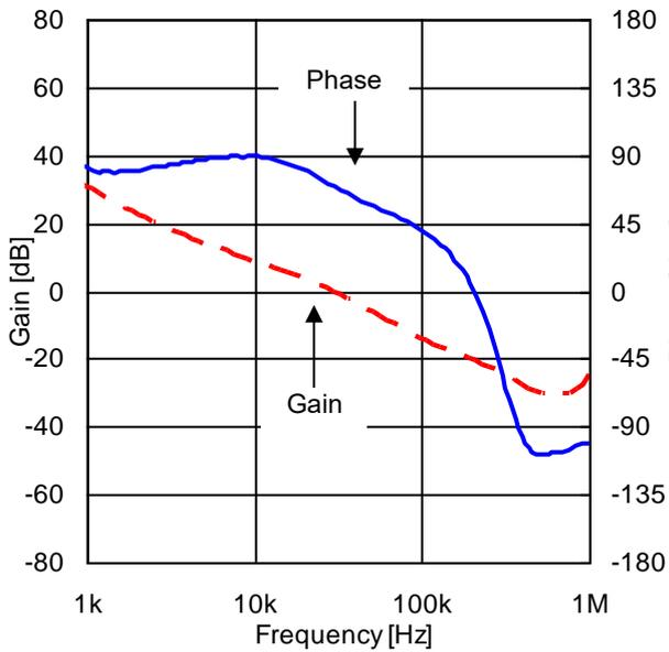
Figure 78. Frequency Characteristic (VIN = 12 V, IOUT = 0.5 A)
