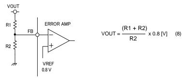
Figure 33. Voltage feed back Resistance Setting Method
