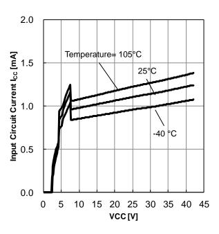
Figure 12. Input Circuit Current vs Input Voltage (V<sub>FB</sub>= 1.2V)
