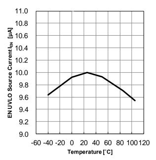
Figure 24. EN Source Current vs Temperature
