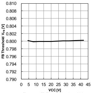
Figure 18. FB Threshold vs Input Voltage
