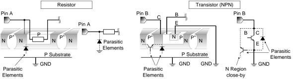
Figure 36. Example of Monolithic IC Structure
