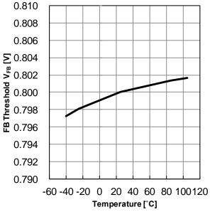
Figure 17. FB Threshold vs Temperature
