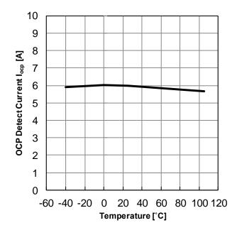
Figure 22. OCP Detect Current vs Temperature
