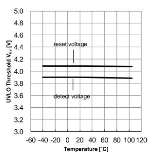
Figure 14. UVLO Threshold vs Temperature
