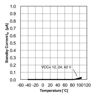
Figure 11. Standby Current vs Temperature
