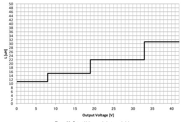
Figure 32. Output Voltage vs inductance (min)
