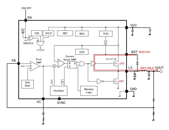
Figure 8. Current Path at the Time of the SW off and Internal REG ON
