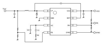
Figure 34. Phase Compensation Element
