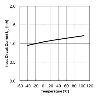
Figure 13. Input Circuit Current vs Temperature (V<sub>FB</sub>= 1.2V)
