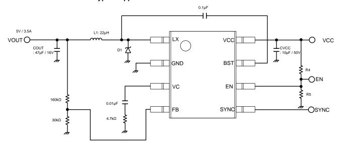
Figure 25. Typical Application Circuits
