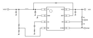
Figure 7. External UVLO Setup
