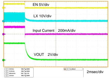
Figure 29. Startup Waveform (IOUT= 0.5A)
