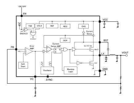
Figure 3. Block Diagram
