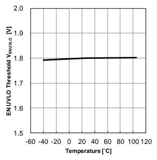
Figure 23. ENUVLO Threshold vs Temperature
