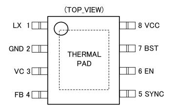
Figure 2. Pin Configuration
