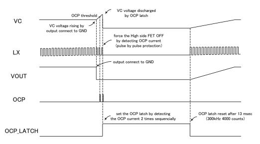
Figure 6. Timing Chart at OCP Operation
