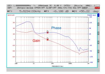
Figure 27. Frequency Characteristics (IOUT= 0.5A)
