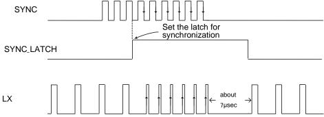
Figure 4. Frequency Synchronization Function Timing Chart
