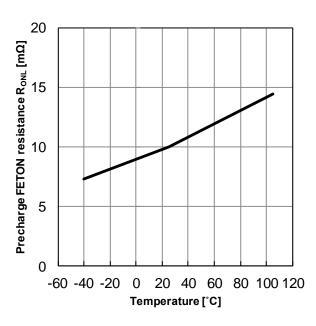
Figure 21. Precharge FET Ron vs Temperature
