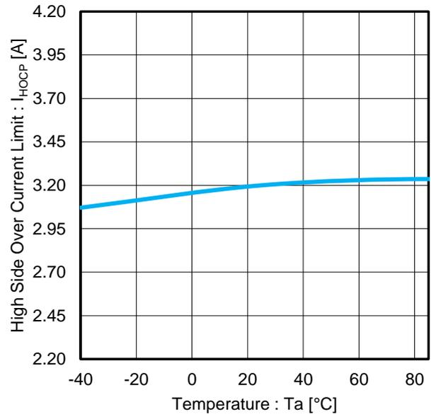
Figure 14. High Side Over Current Limit vs Temperature
