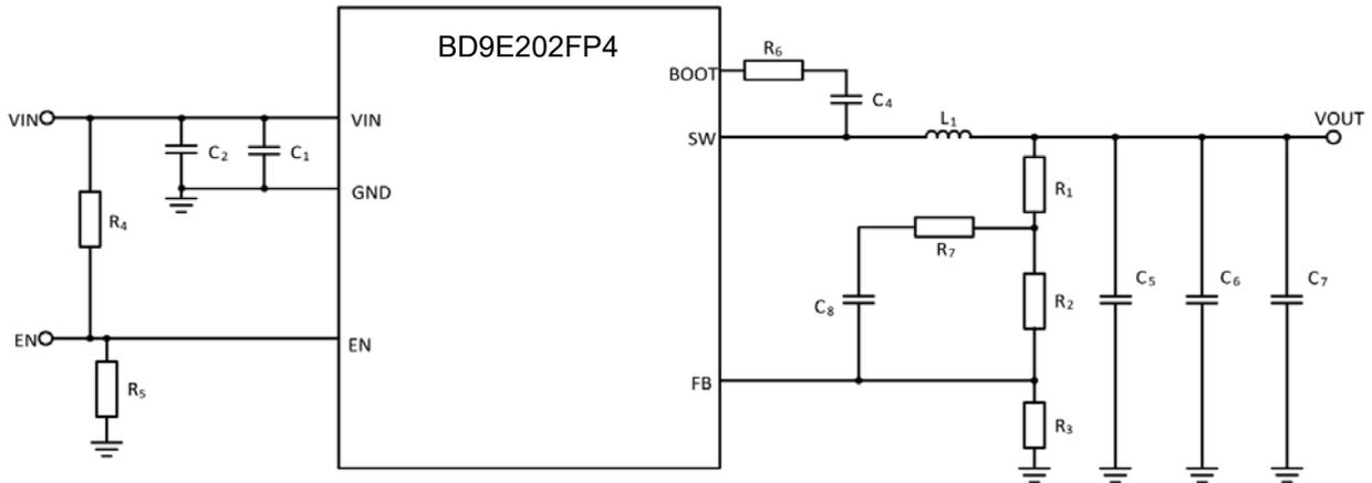
Figure 33. Application Circuit
