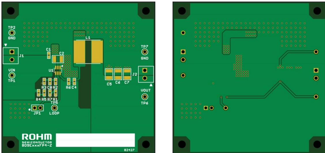
Figure 53. Example of PCB Layout (Silkscreen Overlay)
