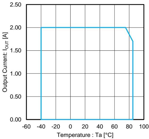
Figure 23. Output Current vs Temperature<sup>(Note 1)</sup> Operating
