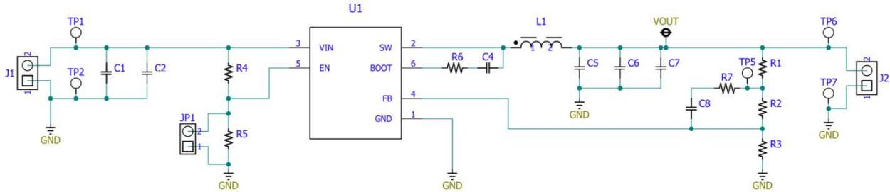
Figure 52. Application Circuit
