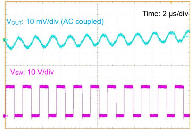
Figure 45. Output Ripple Voltage ( $V_{IN} = 24\text{ V}$ ,  $I_{OUT} = 2\text{ A}$ )
