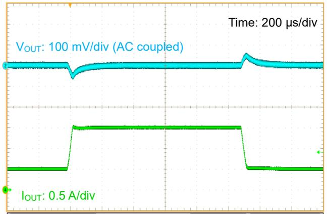
Figure 37. Load Transient Response ( $V_{IN} = 12\text{ V}$ ,  $I_{OUT} = 0.5\text{ A to }1.5\text{ A}$ )
