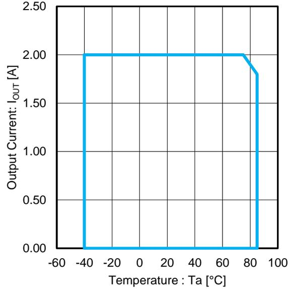
Figure 22. Output Current vs Temperature<sup>(Note 1)</sup>
