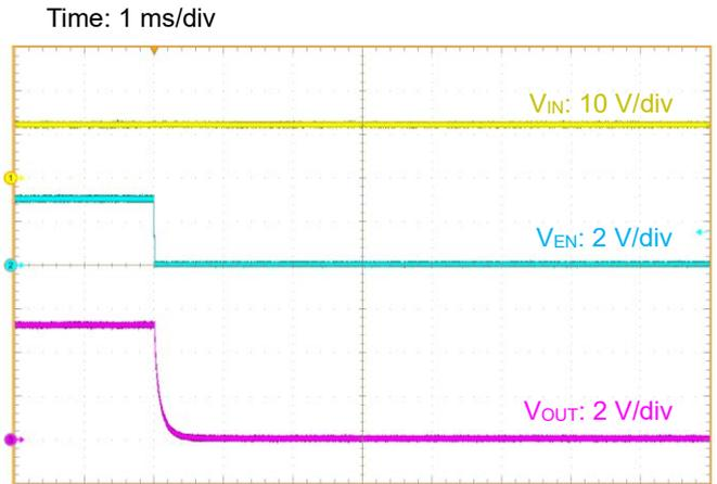
Figure 20. Shutdown at  $R_{LOAD} = 2.5\ \Omega$ :  $V_{EN} = 3\text{ V}$  to  $0\text{ V}$
