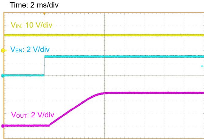
Figure 17. Start-up at No load:  $V_{EN} = 0\text{ V}$  to  $3\text{ V}$
