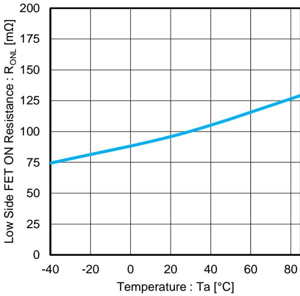
Figure 13. Low Side FET ON Resistance vs Temperature
