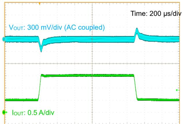
Figure 47. Load Transient Response ( $V_{IN} = 24\text{ V}$ ,  $I_{OUT} = 0.5\text{ A}$  to  $1.5\text{ A}$ )
