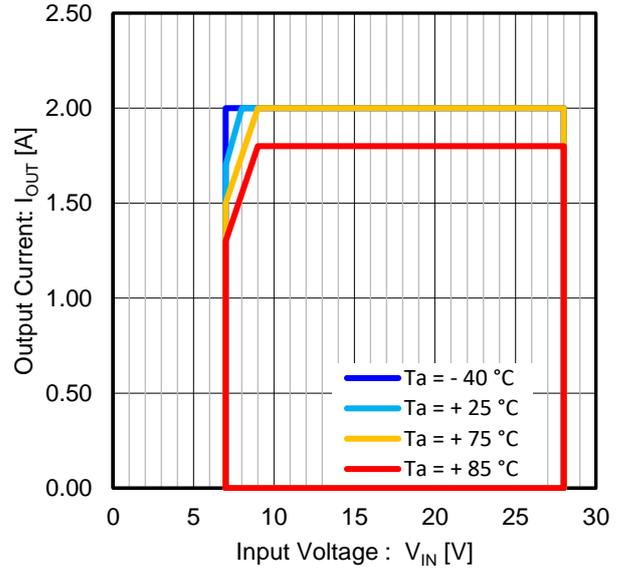
Figure 25. Output Current vs Input Voltage<sup>(Note 1) (Note 2)</sup>
