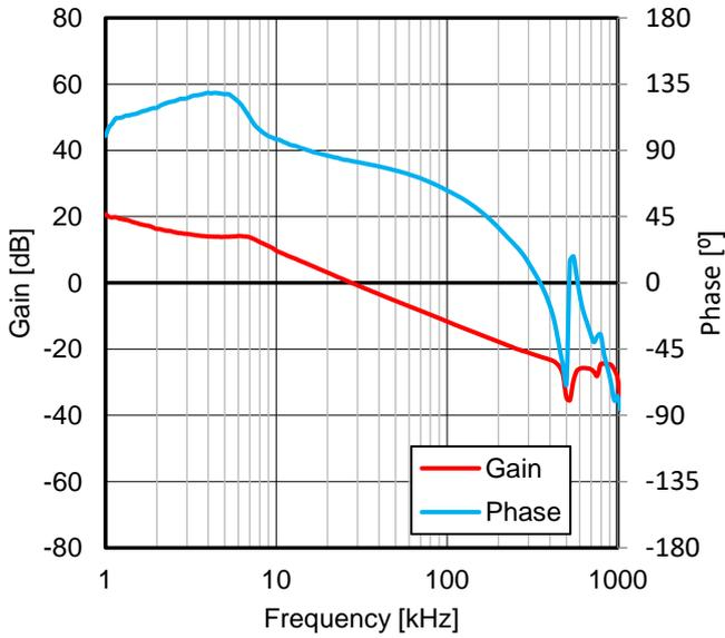
Figure 46. Frequency Characteristics ( $V_{IN} = 24\text{ V}$ ,  $I_{OUT} = 2\text{ A}$ )
