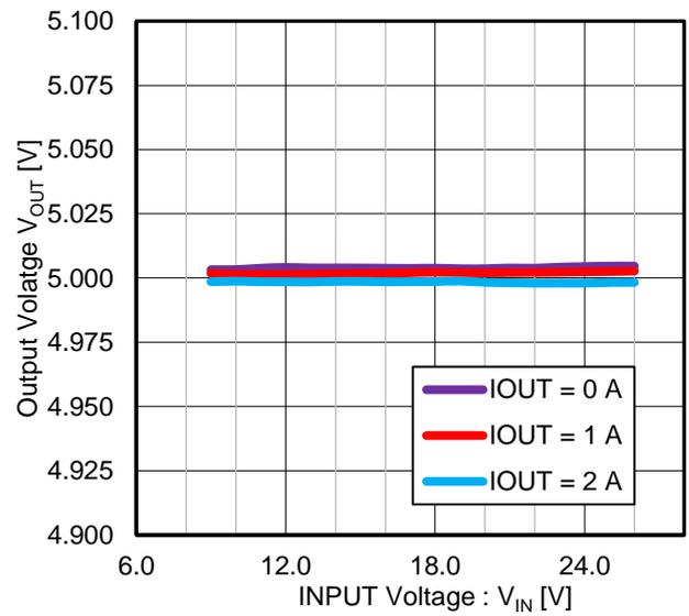
Figure 16. Output Voltage vs Input Voltage
