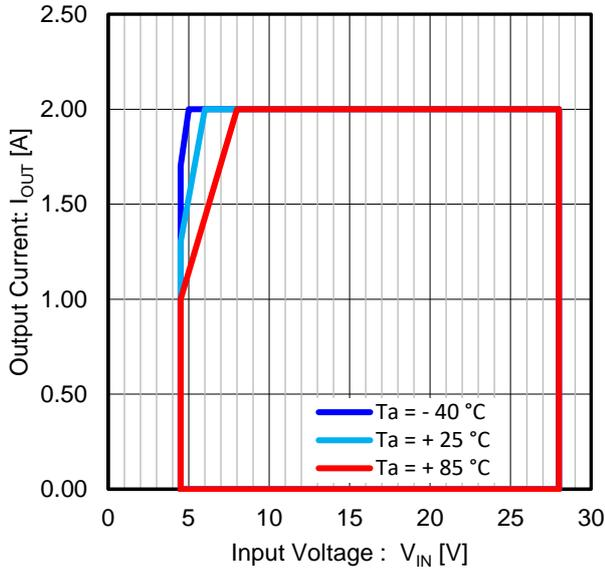
Figure 24. Output Current vs Input Voltage<sup>(Note 1) (Note 2)</sup>
