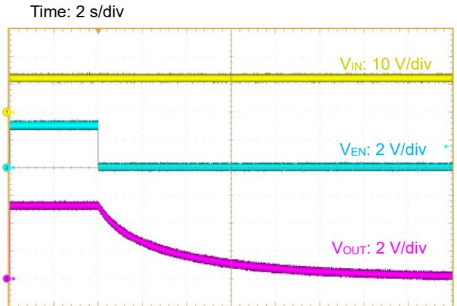
Figure 18. Shutdown at No Load  $V_{EN} = 3\text{ V}$  to  $0\text{ V}$
