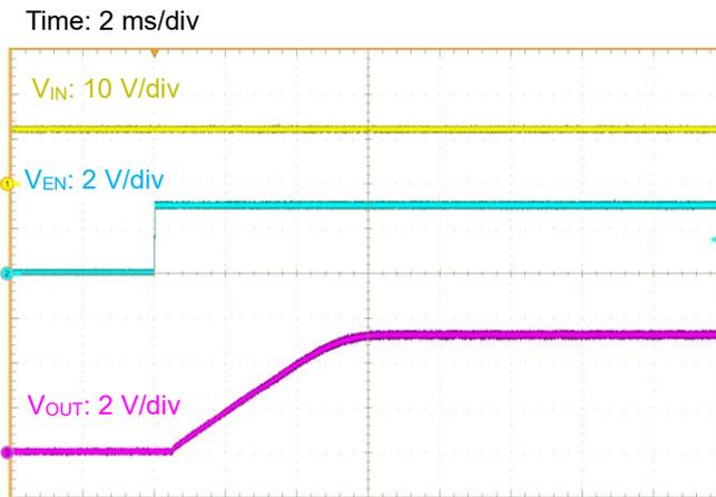
Figure 19. Start-up at  $R_{LOAD} = 2.5\ \Omega$ :  $V_{EN} = 0\text{ V}$  to  $3\text{ V}$
