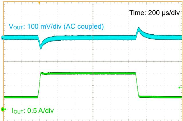
Figure 42. Load Transient Response ( $V_{IN} = 12\text{ V}$ ,  $I_{OUT} = 0.5\text{ A}$  to  $1.5\text{ A}$ )
