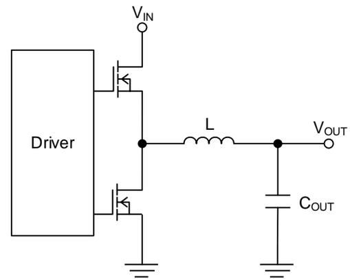
Figure 49. Output LC Filter Circuit
