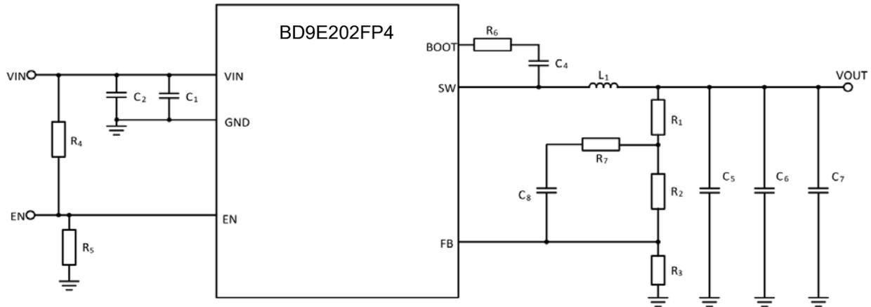
Figure 38. Application Circuit
