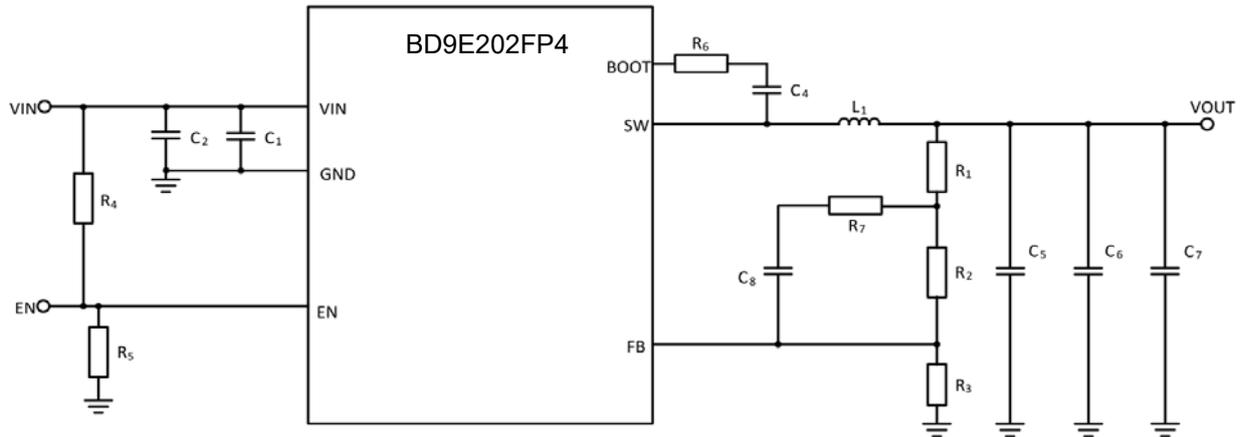
Figure 43. Application Circuit
