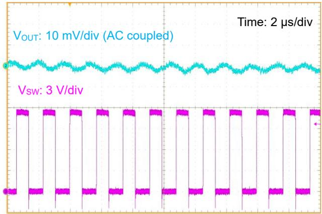
Figure 40. Output Ripple Voltage ( $V_{IN} = 12\text{ V}$ ,  $I_{OUT} = 2\text{ A}$ )
