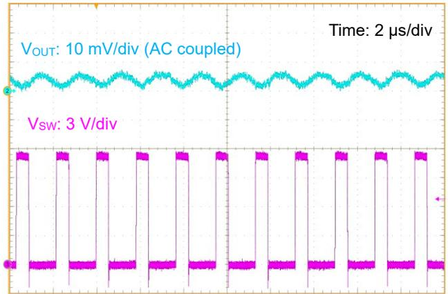
Figure 35. Output Ripple Voltage ( $V_{IN} = 12\text{ V}$ ,  $I_{OUT} = 2\text{ A}$ )
