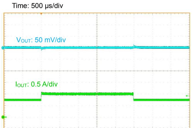
Figure 35. Load Transient Response ( $V_{IN} = 5\text{ V}$ ,  $I_{OUT} = 0.75\text{ A}$  to  $1.0\text{ A}$ )
