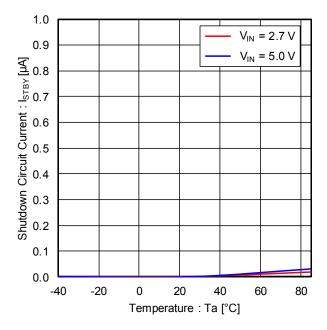
Figure 1. Shutdown Current vs Temperature
