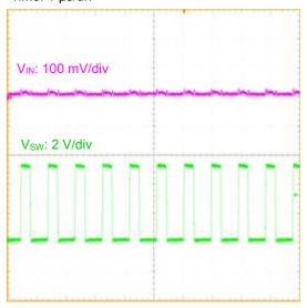
Figure 19. Input Voltage Ripple (V<sub>IN</sub> = 5 V, V<sub>OUT</sub> = 1.8 V, I<sub>OUT</sub> = 0 A)
