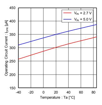
Figure 2. Operating Circuit Current vs Temperature
