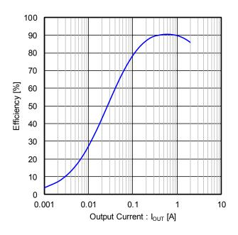
Figure 31. Efficiency vs Output Current
