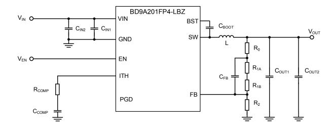
Figure 25. Application Circuit
