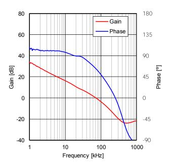
Figure 38. Frequency Characteristics ( $I_{OUT} = 1 A$ )
