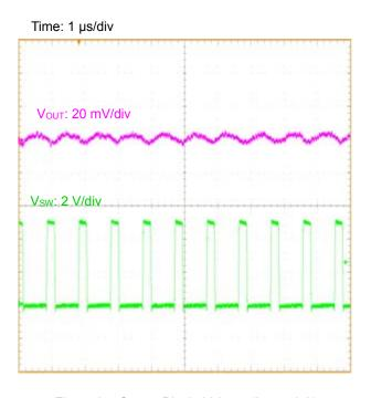
Figure 37. Output Ripple Voltage (Iout = 2 A)
