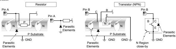
Figure 44. Example of Monolithic IC Structure
