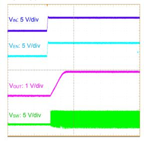
Figure 13. Start-up at R<sub>LOAD</sub> = 0.9  $\Omega$  (V<sub>EN</sub> = V<sub>IN</sub>, V<sub>IN</sub> = 5 V, V<sub>OUT</sub> = 1.8 V)
