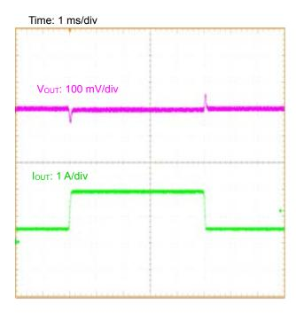
Figure 29. Load Transient Response (I<sub>OUT</sub> = 0.5 A to 2.0 A)
