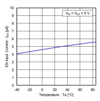
Figure 12. EN Input Current vs Temperature
