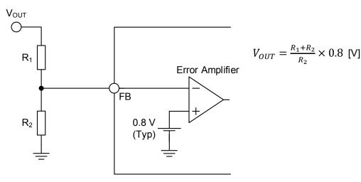
Figure 42. Feedback Resistor Circuit
