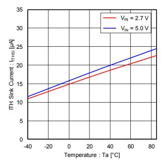
Figure 5. ITH Sink Current vs Temperature
