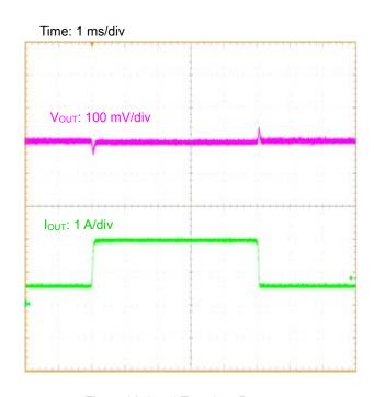
Figure 39. Load Transient Response (I<sub>OUT</sub> = 0.5 A to 2.0 A)
