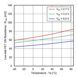
Figure 9. Low-side FET ON Resistance vs Temperature
