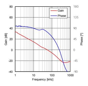
Figure 28. Frequency Characteristics (I<sub>OUT</sub> = 1 A)
