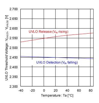
Figure 10. UVLO Threshold Voltage vs Temperature
