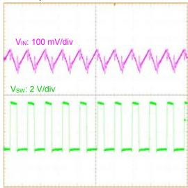
Figure 20. Input Voltage Ripple (V<sub>IN</sub> = 5 V, V<sub>OUT</sub> = 1.8 V, I<sub>OUT</sub> = 2 A)
