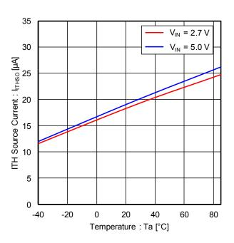
Figure 6. ITH Source Current vs Temperature
