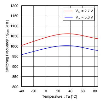
Figure 3. Switching Frequency vs Temperature
