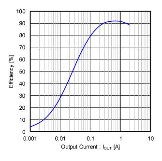
Figure 26. Efficiency vs Output Current
