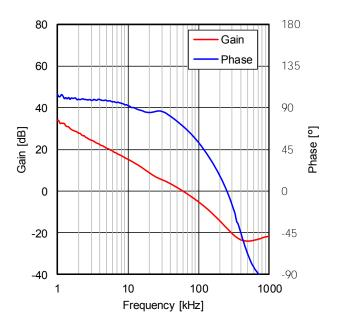
Figure 33. Frequency Characteristics (I<sub>OUT</sub> = 1 A)
