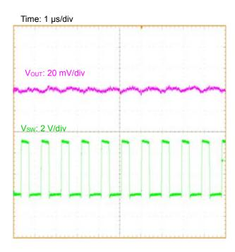
Figure 27. Output Ripple Voltage (Iout = 2 A)
