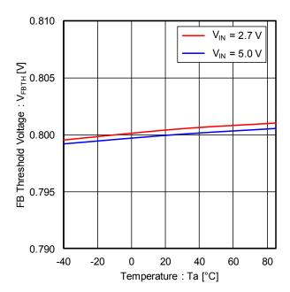
Figure 4. FB Threshold Voltage vs Temperature
