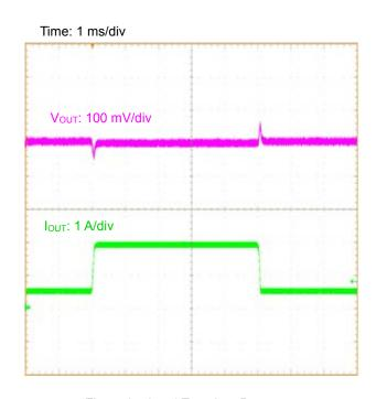
Figure 34. Load Transient Response (I<sub>OUT</sub> = 0.5 A to 2.0 A)
