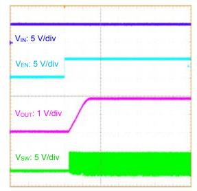
Figure 15. Start-up at  $R_{LOAD}$  = 0.9  $\Omega$  ( $V_{EN}$  = 0 V to 5 V,  $V_{IN}$  = 5 V,  $V_{OUT}$  = 1.8 V)
