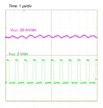
Figure 32. Output Ripple Voltage (Iout = 2 A)
