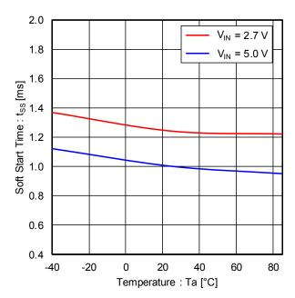
Figure 7. Soft Start Time vs Temperature
