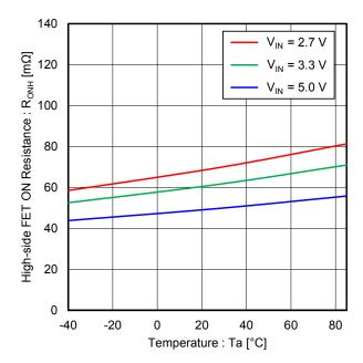
Figure 8. High-side FET ON Resistance vs Temperature
