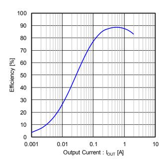
Figure 36. Efficiency vs Output Current
