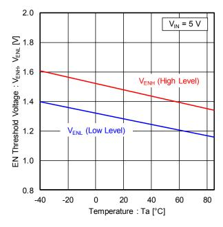
Figure 11. EN Threshold Voltage vs Temperature
