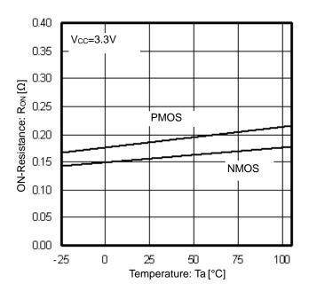
Figure 10. ON-Resistance vs Temperature
