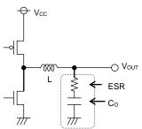
Figure 27. Output Capacitor
