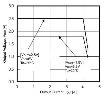
Figure 6. Output Voltage vs Output Current
