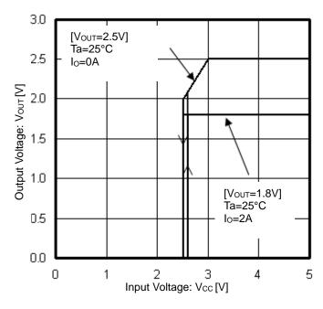
Figure 4. Output Voltage vs Input Voltage
