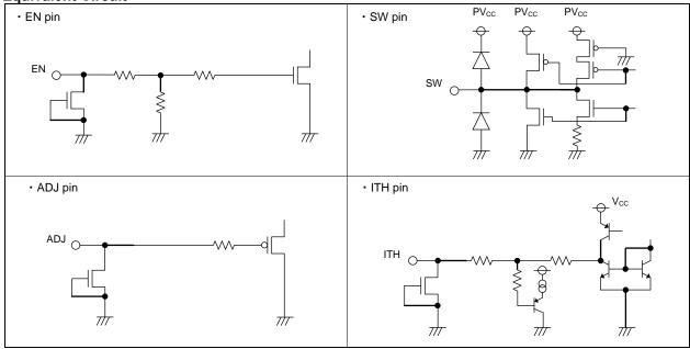
Figure 35. I/O Equivalent Circuit
