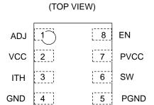
Figure 2. Pin Configuration
