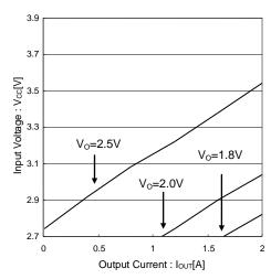
Figure 33. Minimum Input Voltage in each Output Voltage
