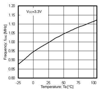
Figure 9. Frequency vs Temperature
