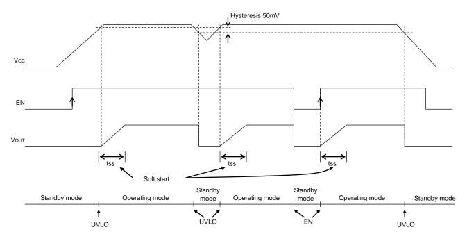
Figure 20. Soft Start, Shutdown, UVLO Timing Chart
