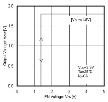
Figure 5. Output Voltage vs EN Voltage
