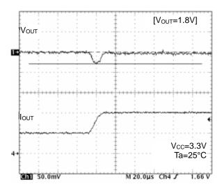
Figure 16. Transient Response ( $I_0$ =1A to 2A, 10 $\mu$ s)
