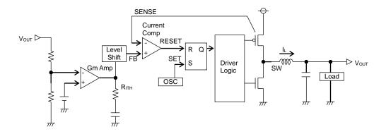
Figure 18. Diagram of Current Mode PWM Control
