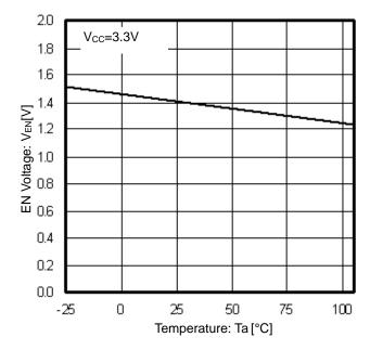
Figure 11. EN Voltage vs Temperature
