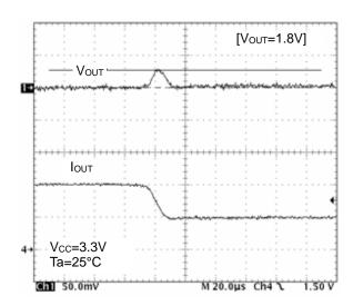
Figure 17. Transient Response (Io=2A to 1A, 10µs)
