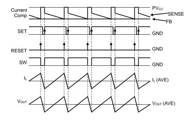
Figure 19. PWM Switching Timing Chart
