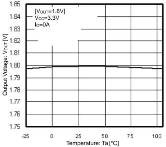
Figure 7. Output Voltage vs Temperature
