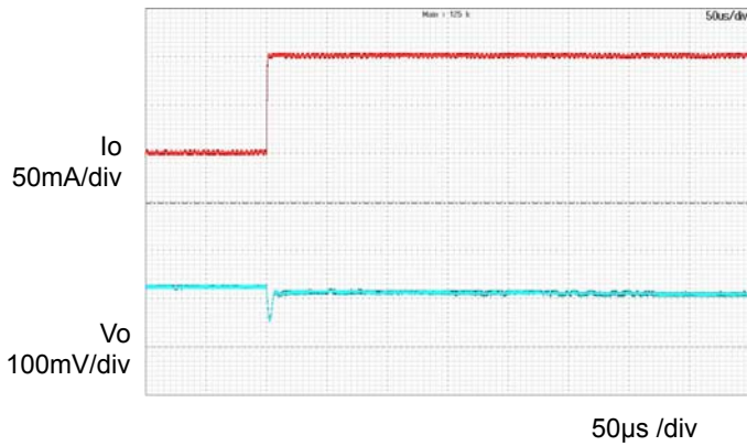
Figure 12. Transient Response ( T_a=105^{\circ}\text{C} ) ( I_o = 0\text{A} \rightarrow 0.1\text{A} )
