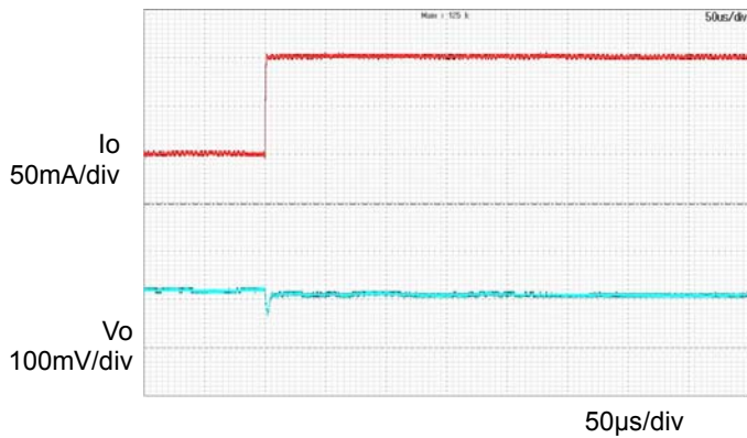
Figure 8. Transient Response ( T_a=25^\circ\text{C} ) ( I_o = 0\text{A}\rightarrow 0.1\text{A} )
