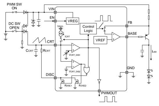
Figure 14. PWM Dimming Operation
