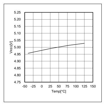
Figure 3.  $V_{\text{REG}}$  vs Temp
