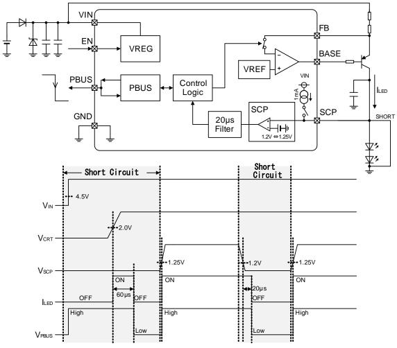
Figure 21. Short Circuit Protection (SCP)
