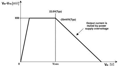
Figure 27. Overvoltage Mute Function (OVM)
