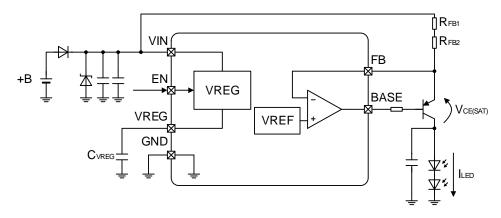
Figure 13. LED Current Setting
