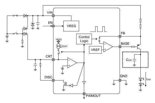
Figure 23. About the capacitor of connecting LED anode
