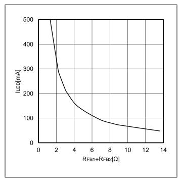
Figure 4.  $I_{LED}$  vs  $R_{FB1}$ + $R_{FB2}$
