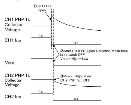
Figure 26. Example of Protective Operation
