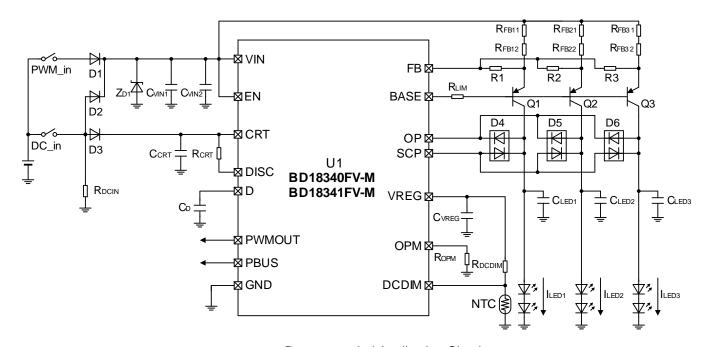
Figure 32. Recommended Application Circuit 4 (ILED1~3 120mA, LED white 2strings×3, PWM ON Duty: 10%( pulse width: 0.334ms), PWM frequency: 300Hz)
