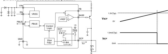
Figure 22. SCP Terminal Source Current
