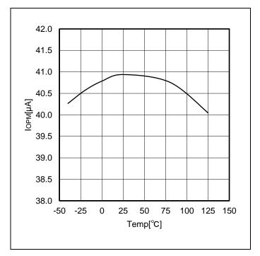
Figure 12.  $I_{\text{OPM}}$  vs Temp
