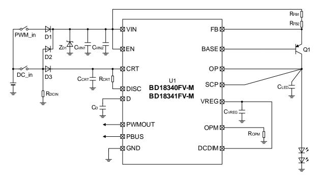
Figure 30. Recommended Application Circuit 2 (ILED 120mA, LED white 2strings, PWM ON Duty: 10%(Pulse width: 0.334ms), PWM frequency: 300Hz)
