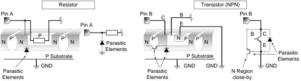
Figure 33. Example of monolithic IC structure
