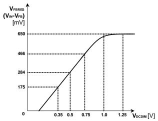
Figure 24. LED Current De-rating Function (DC Dimming Function)
