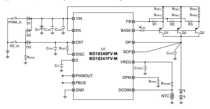
Figure 31. Recommended Application Circuit 3 (I<sub>LED</sub> 542mA, LED white 2strings, PWM ON Duty: 10%(pulse width: 0.334ms), PWM frequency: 300Hz)
