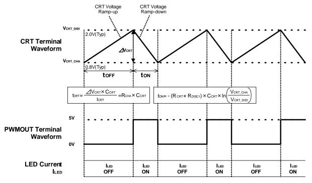
Figure 15. PWM Dimming Operation
