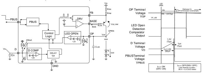
Figure 18. LED Open Detection Timing Chart
