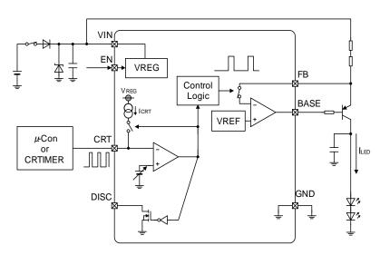
Figure 16. PWM Dimming Operation using external signal
