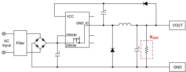
Figure 9. Location of Resistor ROUT
