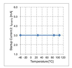
Figure 34. Startup Current 2 vs Temperature
