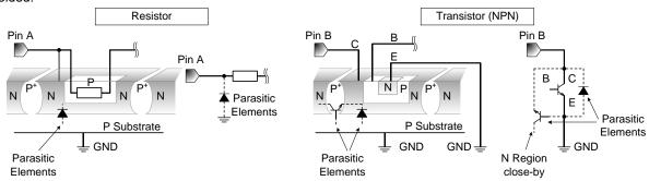
Figure 35. Example of IC Structure
