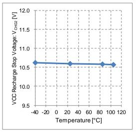
Figure 27. VCC Recharge Stop Voltage vs Temperature (BM2P131X-Z, BM2P141X-Z, BM2P151X-Z, BM2P161X-Z, BM2P181X-Z, BM2P201X-Z, BM2P241X-Z)
