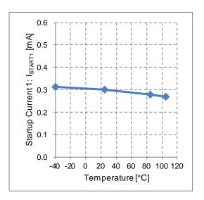
Figure 33. Startup Current 1 vs Temperature
