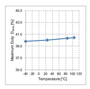
Figure 29. Maximum Duty vs Temperature
