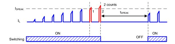
Figure 12. Dynamic Over Current Limiter
