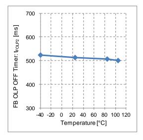
Figure 31. FB OLP OFF Timer vs Temperature
