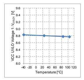
Figure 18. VCC UVLO Voltage 1 vs Temperature (BM2P101X-Z, BM2P121X-Z)
