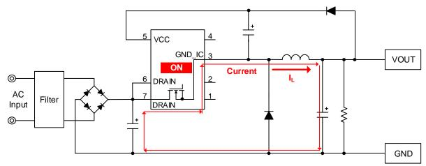
Figure 1. Back Converter Operation (MOSFET = ON)
