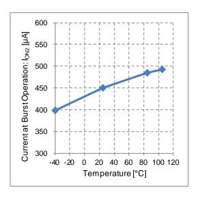
Figure 17. Current at Burst Operation vs Temperature
