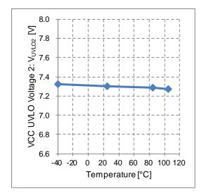
Figure 20. VCC UVLO Voltage 2 vs Temperature (BM2P101X-Z, BM2P121X-Z)
