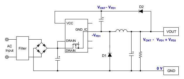
Figure 8. Back Converter Circuit (MOSFET = OFF)
