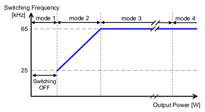
Figure 11. State Transition of Switching Frequency
