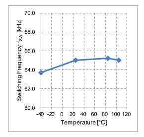
Figure 28. Switching Frequency vs Temperature
