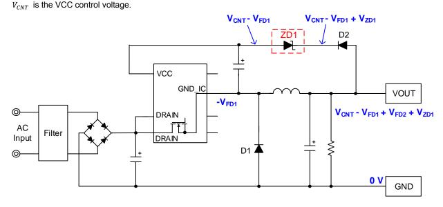
Figure 10. Back Converter Output Dispersion Circuit (MOSFET = OFF)
