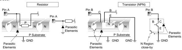
Figure 33. Example of IC Structure
