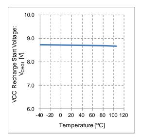
Figure 21. VCC Recharge Start Voltage vs Temperature
