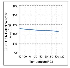
Figure 28. FB OLP ON Detection Timer vs Temperature
