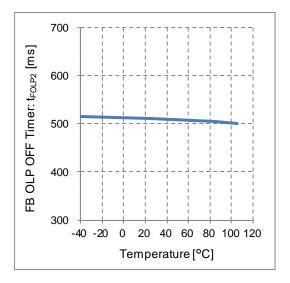
Figure 29. FB OLP OFF Timer vs Temperature
