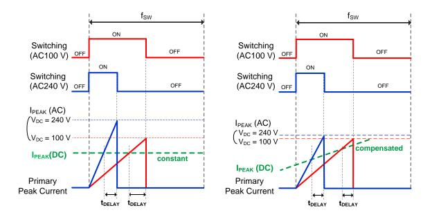
Figure 8. Without the AC Voltage Compensation Function
