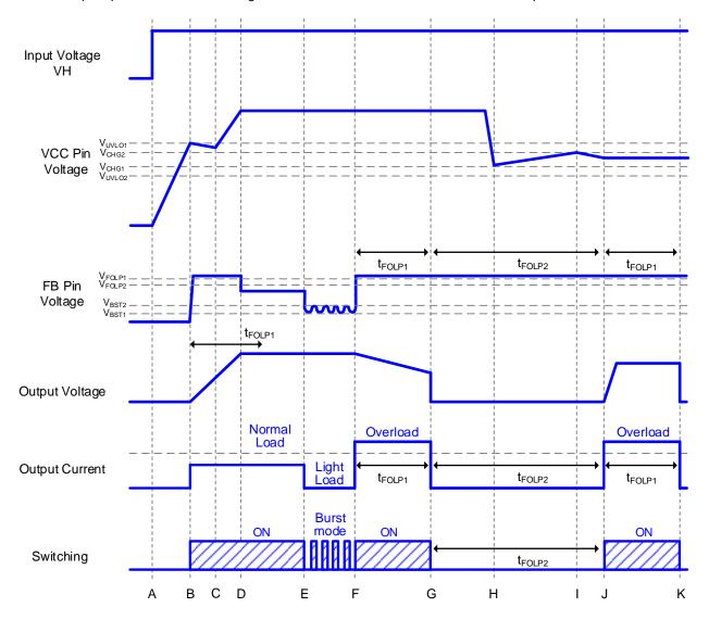
Figure 4. Startup Sequences Timing Chart
