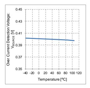
Figure 30. Over Current Detection Voltage vs Temperature
