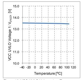
Figure 15. VCC UVLO Voltage 1 vs Temperature
