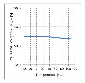
Figure 19. VCC OVP Voltage 2 vs Temperature
