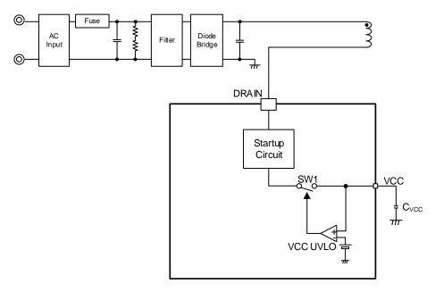
Figure 1. Block Diagram of Startup Circuit
