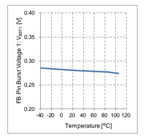
Figure 25. FB Pin Burst Voltage 1 vs Temperature
