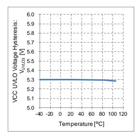
Figure 17. VCC UVLO Voltage Hysteresis vs Temperature
