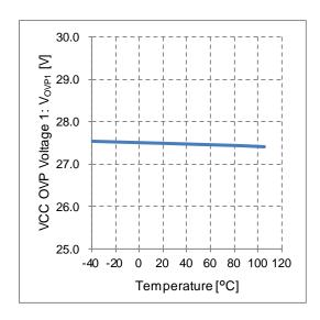
Figure 18. VCC OVP Voltage 1 vs Temperature
