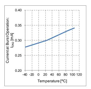
Figure 14. Current at Burst Operation vs Temperature
