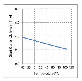
Figure 32. Start Current 2 vs Temperature
