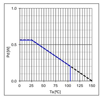
Figure 12. SOP8 Thermal Dissipation Characteristic
