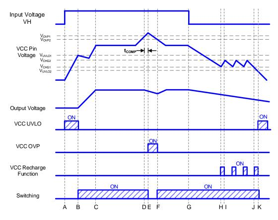
Figure 5. VCC UVLO/VCC OVP/VCC Recharge Function Timing Chart
