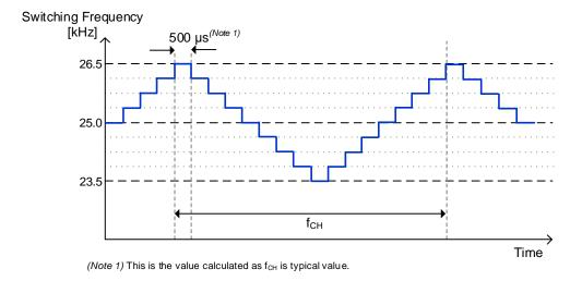
Figure 6. Frequency Hopping Function
