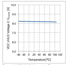
Figure 16. VCC UVLO Voltage 2 vs Temperature
