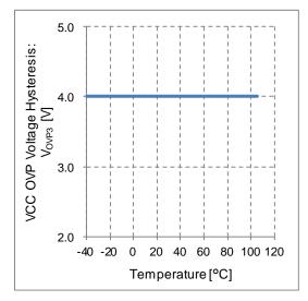
Figure 20. VCC OVP Voltage Hysteresis vs Temperature
