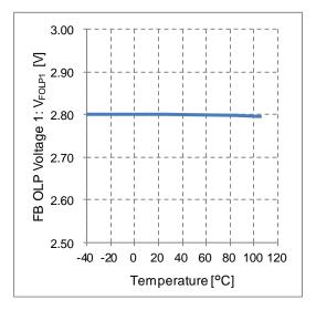
Figure 27. FB OLP Voltage 1 vs Temperature
