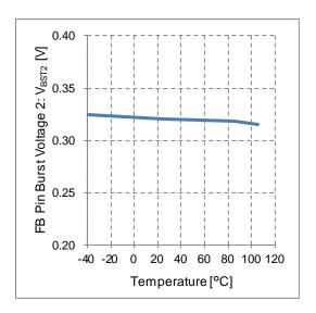
Figure 26. FB Pin Burst Voltage 2 vs Temperature
