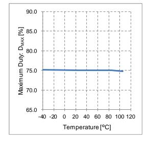
Figure 24. Maximum Duty vs Temperature
