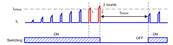
Figure 11. Dynamic Over Current Limiter
