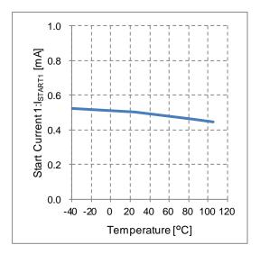
Figure 31. Start Current 1 vs Temperature
