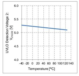
Figure 11. UVLO Detection Voltage 2 vs Temperature
