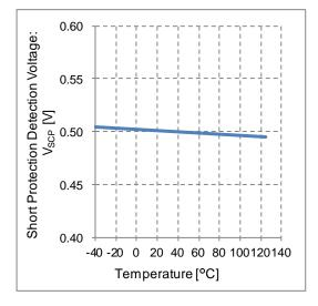
Figure 27. Short Protection Detection Voltage vs Temperature
