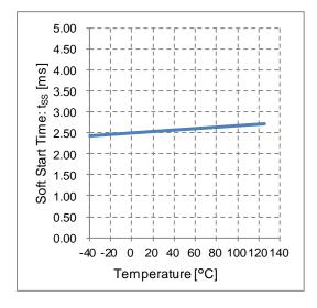
Figure 26. Soft Start Time vs Temperature
