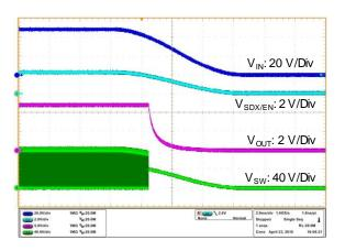
Figure 41. Shutdown Waveform (The VIN Pin Control)
