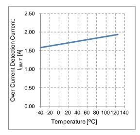
Figure 20. Over Current Detection Current vs Temperature
