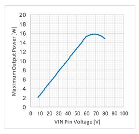
Figure 43. Maximum Output Power vs VIN Pin Voltage
