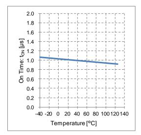
Figure 22. On Time vs Temperature
