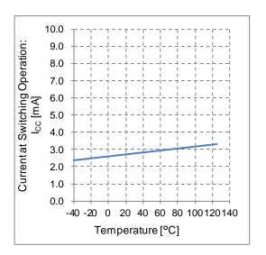
Figure 9. Current at Switching Operation vs Temperature
