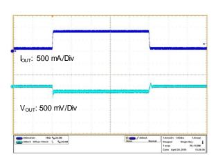
Figure 42. Load Transient Response (I<sub>OUT</sub> = 0.1 A to 0.83 A)
