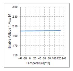
Figure 14. Enable Voltage 1 vs Temperature
