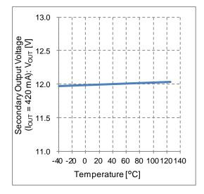
Figure 34. Secondary Output Voltage vs Temperature (I<sub>OUT</sub> = 420 mA)
