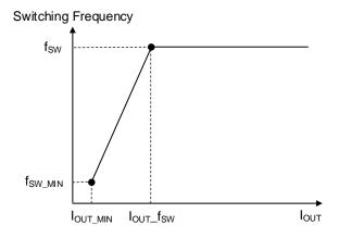
Figure 48. Switching Frequency vs IOUT
