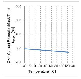
Figure 30. Over Current Protection Mask Time vs Temperature
