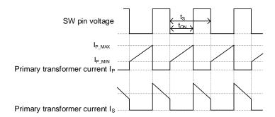
Figure 50. Switching Operation or Continuous Mode
