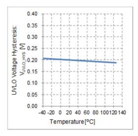
Figure 12. UVLO Voltage Hysteresis vs Temperature
