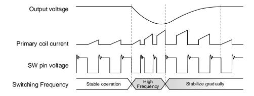
Figure 3. Transient Response Timing Chart
