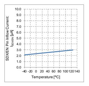
Figure 17. SDX/EN Pin Inflow Current vs Temperature
