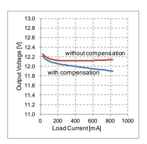
Figure 37. Output Voltage vs Load Current
