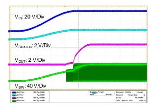
Figure 40. Startup Waveform (The VIN Pin Control)
