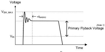
(Note 1) Primary Flyback Voltage =  $\frac{N_P}{N_S} \times (V_{OUT} + V_F + I_S \times ESR)$
