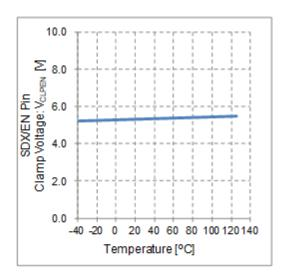
Figure 13. SDX/EN Pin Clamp Voltage vs Temperature
