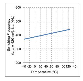
Figure 35. Switching Frequency vs Temperature (I<sub>OUT</sub> = 420 mA)
