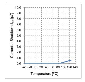
Figure 8. Current at Shutdown vs Temperature
