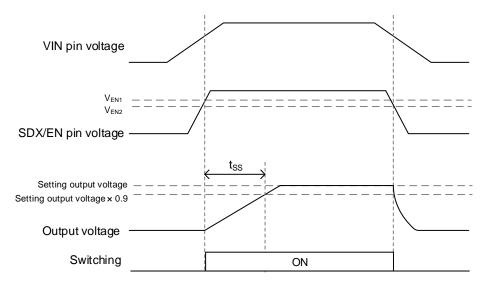
Figure 1. Startup and Stop Timing Chart
