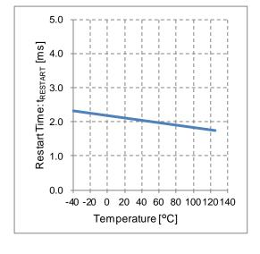
Figure 33. Restart Time vs Temperature
