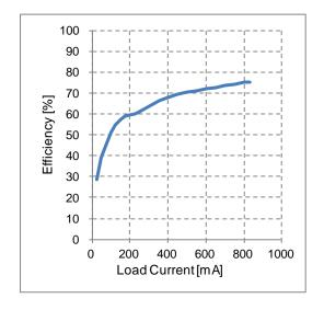
Figure 36. Efficiency vs Load Current
