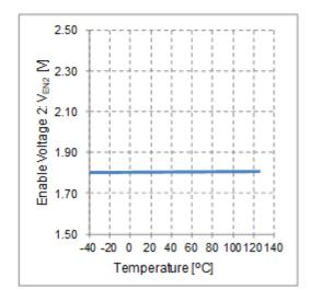
Figure 15. Enable Voltage 2 vs Temperature
