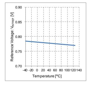
Figure 18. Reference Voltage vs Temperature
