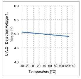
Figure 10. UVLO Detection Voltage 1 vs Temperature
