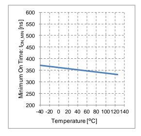
Figure 23. Minimum On Time vs Temperature
