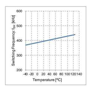
Figure 21. Switching Frequency vs Temperature
