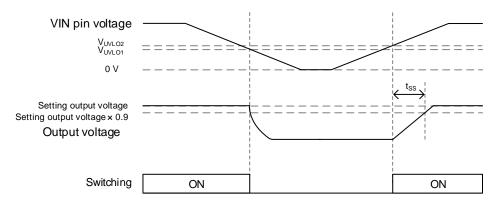
Figure 2. VIN UVLO Timing Chart
