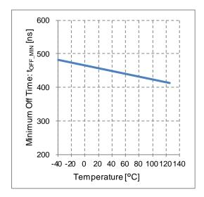
Figure 24. Minimum Off Time vs Temperature
