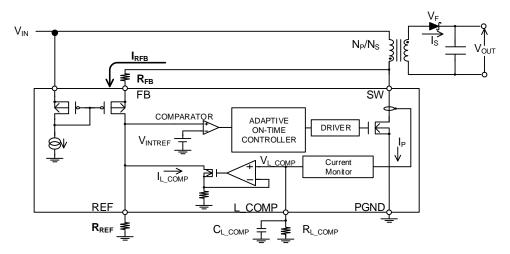
Figure 44. Control Block Diagram
