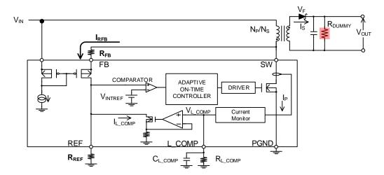
Figure 47. Position of  $R_{\text{DUMMY}}$
