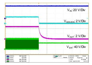
Figure 39. Shutdown Waveform (The SDX/EN Pin Control)
