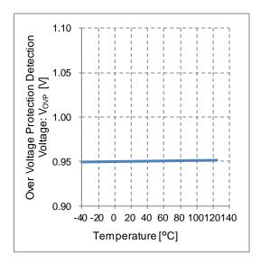
Figure 28. Over Voltage Protection Detection Voltage vs Temperature
