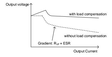
Figure 51. Image of Load Compensation
