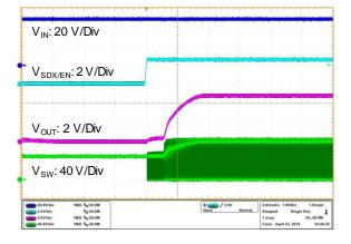
Figure 38. Startup Waveform (The SDX/EN Pin Control)
