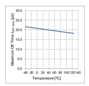
Figure 25. Maximum Off Time vs Temperature
