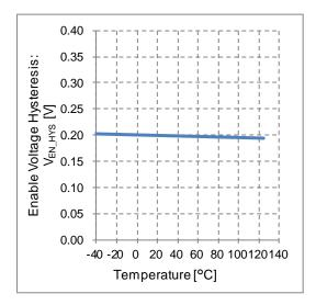
Figure 16. Enable Voltage Hysteresis vs Temperature
