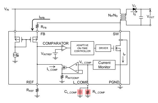
Figure 49. Block Diagram of Load Compensation
