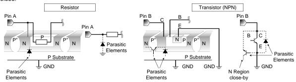
Figure 52. Example of Monolithic IC Structure
