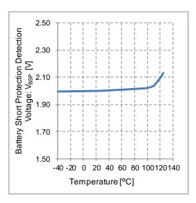
Figure 29. Battery Short Protection Detection Voltage vs Temperature
