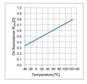
Figure 19. On Resistance vs Temperature
