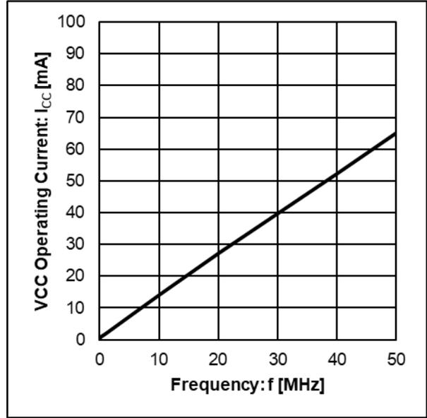
Figure 2. VCC Operating Current vs Frequency
