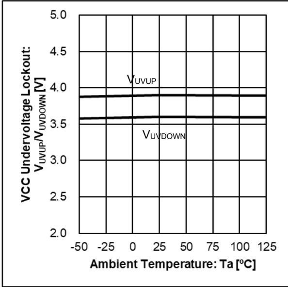
Figure 1. VCC Undervoltage Lockout vs Ambient Temperature
