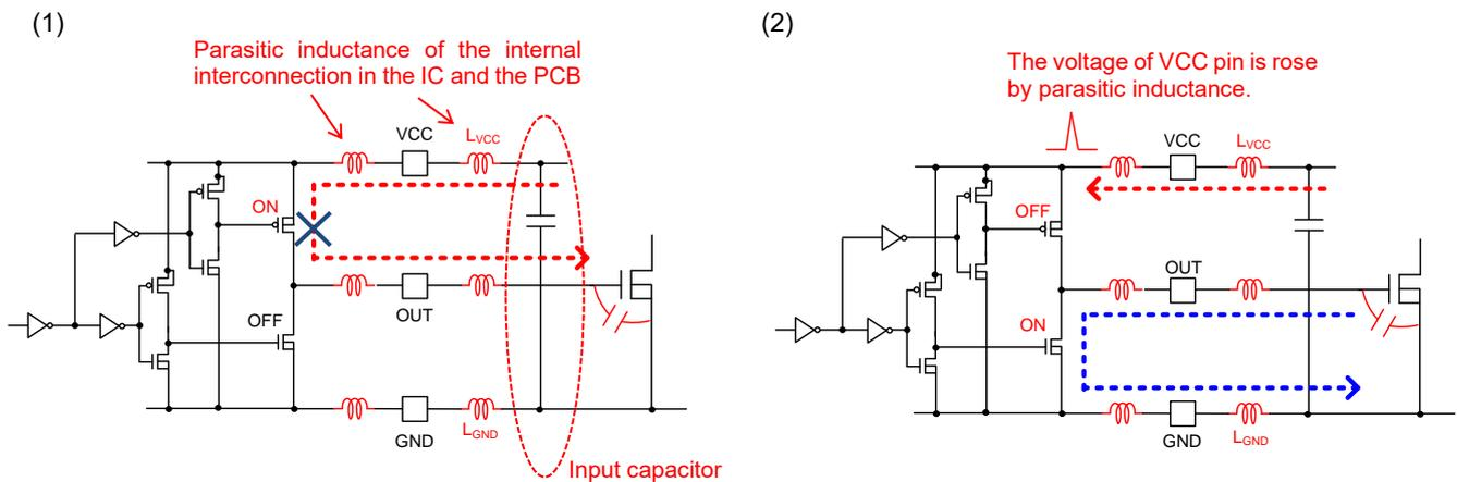
Figure 15. Mechanism of Overshoot
