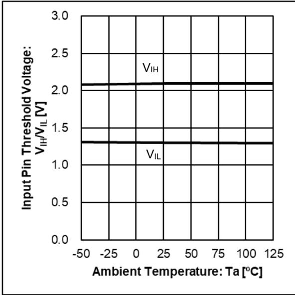
Figure 5. Input Pin Threshold Voltage vs Ambient Temperature
