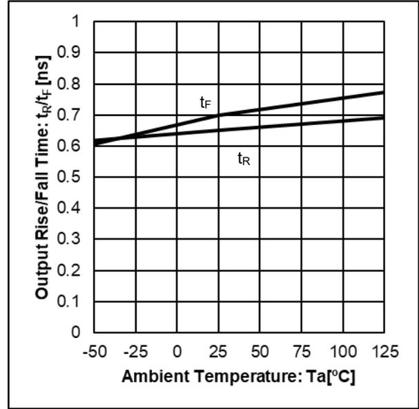
Figure 6. Output Rise/Fall Time vs Ambient Temperature
