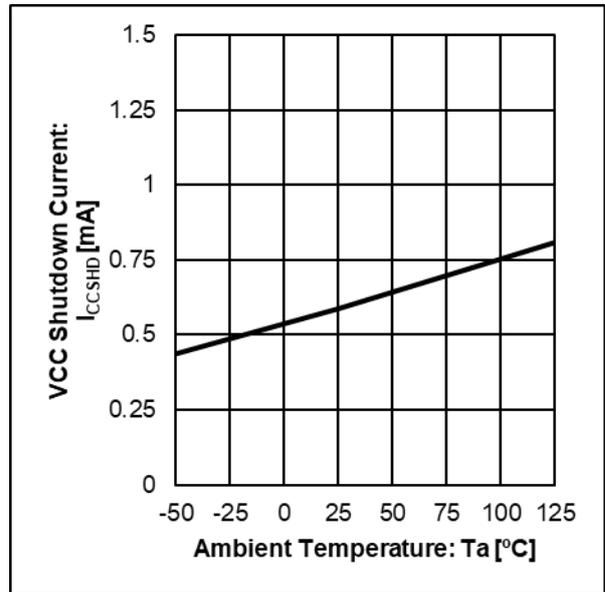
Figure 4. VCC Shutdown Current vs Ambient Temperature
