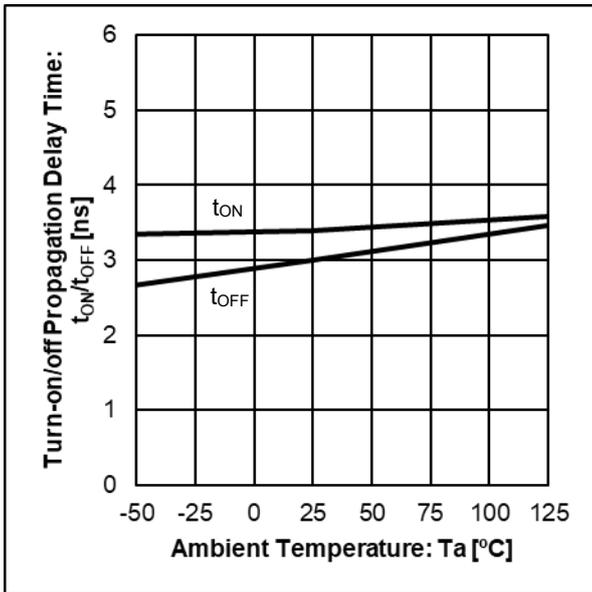
Figure 7. Turn-on/off Propagation Delay Time vs Ambient Temperature
