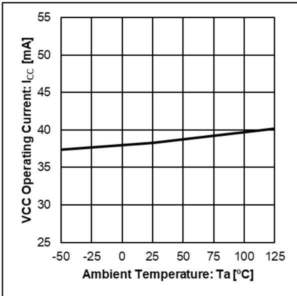
Figure 3. VCC Operating Current vs Ambient Temperature
