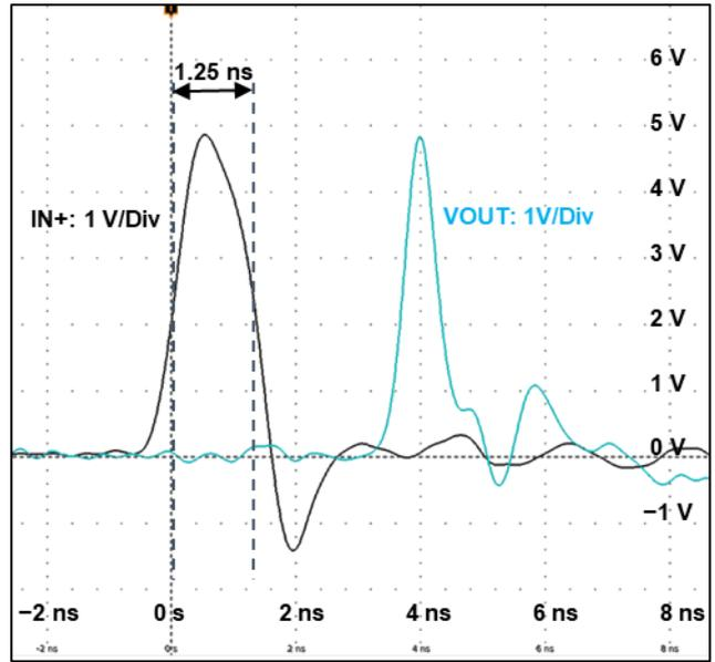
Figure 10. Minimum Input Pulse Width
