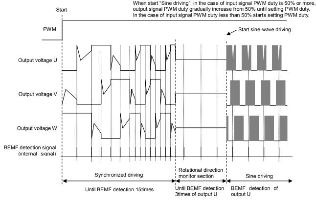
Figure 18. Timing chart at startup
