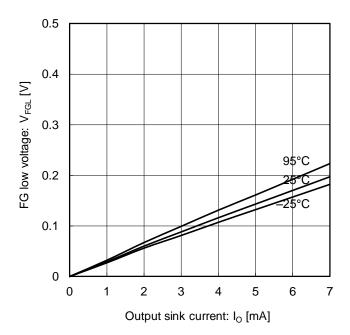
Figure 9. FG low voltage (V<sub>CC</sub>=5V)
