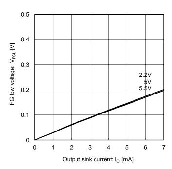
Figure 10. FG low voltage (Temp=25°C)
