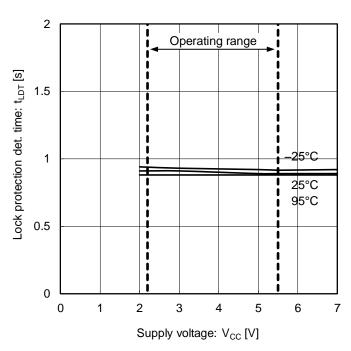
Figure 16. Lock protection det.time
