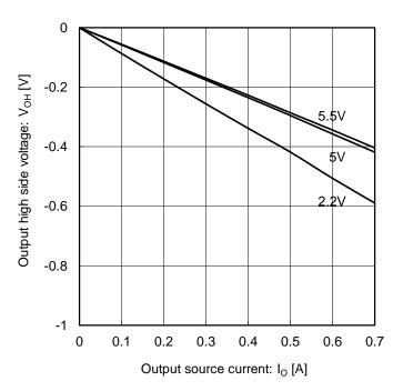
Figure 12. Output high side voltage (Temp=25°C)
