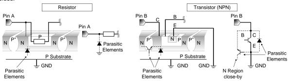
Figure 34. Example of Monolithic IC Structure
