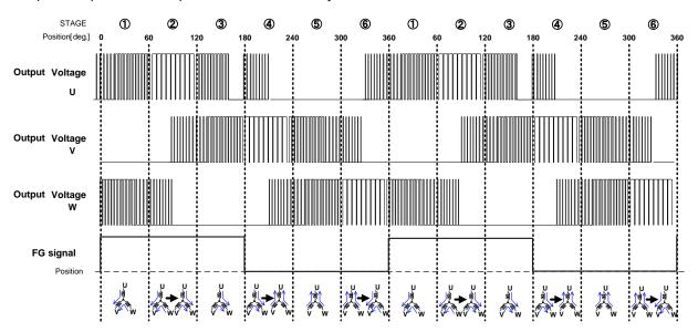
Figure 20. Timing chart of U, V, W, FG output signal (FR= Hi or no connect)
