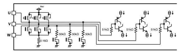
Figure 33. I/O equivalent circuits
