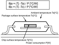
Figure 25. Thermal resistance
