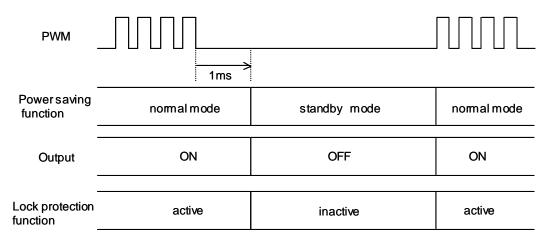
Figure 23. The power saving function
