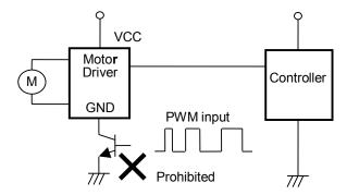
Figure 30. GND Line PWM switching prohibited
