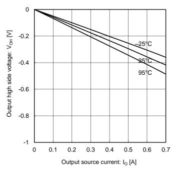
Figure 11. Output high side voltage (V<sub>CC</sub>=5V)
