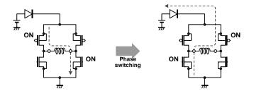
Figure 28. VCC voltage rise by back electromotive force
