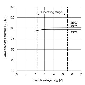
Figure 8. TOSC discharge current
