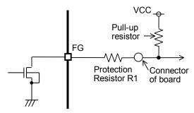
Figure 31. Protection of FG terminal
