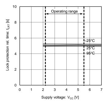
Figure 17. Lock protection rel.time
