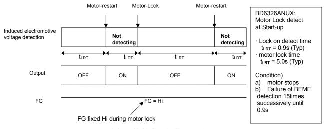
Figure 22. Lock protection operation
