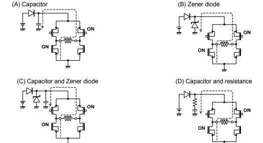
Figure 29. Measure against VCC voltage rise
