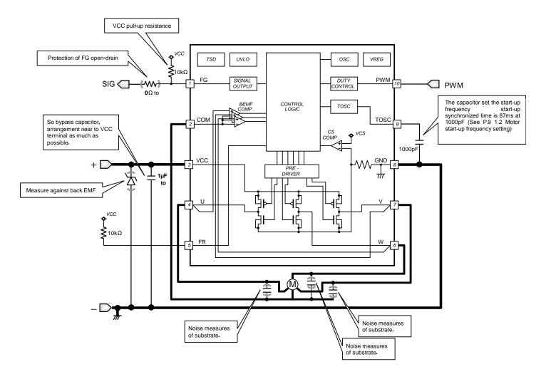
Figure 24. PWM controllable 4 wires type (FG) motor application circuit
