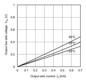
Figure 13. Output low side voltage ( $V_{\text{CC}}$ =5V)
