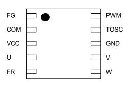
Figure 1. Pin configuration
