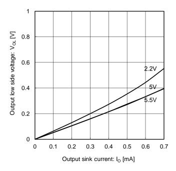
Figure 14. Output low side voltage (Temp=25°C)
