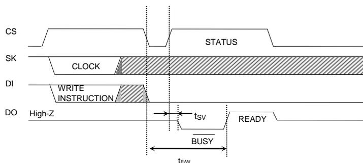
Figure 48. READY/ $\overline{\text{BUSY}}$  STATUS output timing chart
