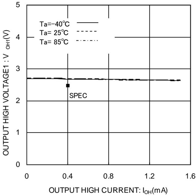
Figure 8. Output high voltage1 V<sub>OH1</sub>(VCC=2.7V)
