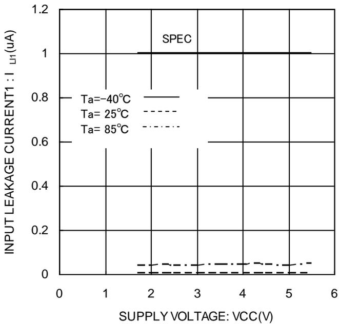
Figure 10. Input leakage current1 I<sub>LI1</sub>(CS,SK,DI)
