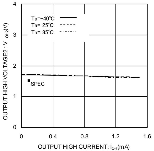
Figure 9. Output high voltage2 V<sub>OH2</sub>(VCC=1.7V)
