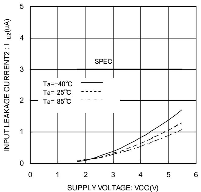
Figure 11. Input leakage current2 I<sub>LI2</sub>(ORG)
