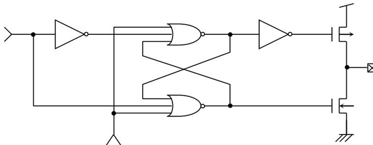
Figure 61. Output Equivalent Circuit (SO)
