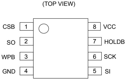
Figure 3-(a). Pin Configuration (SOP-J8, TSSOP-B8, MSOP8)
