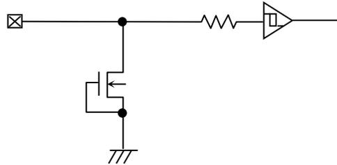
Figure 60. Input Equivalent Circuit (CSB, SCK, SI, HOLDB, WPB)
