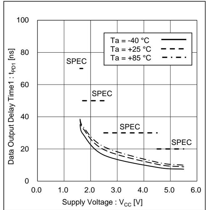
Figure 28. Data Output Delay Time1 vs Supply Voltage
