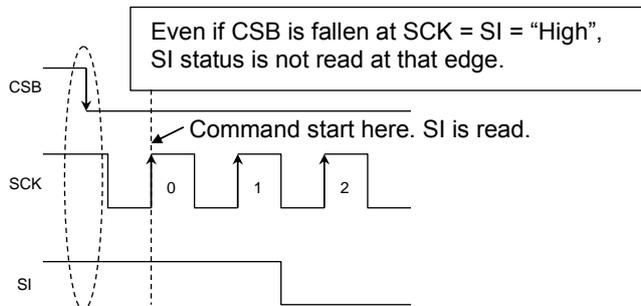
Figure 51. Operating Timing
