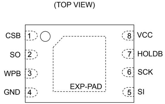
Figure 3-(b). Pin Configuration (VSON008X2030)
