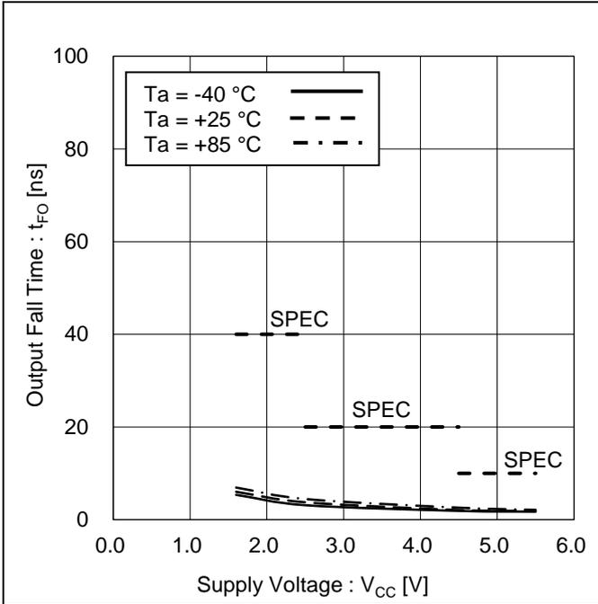
Figure 35. Output Fall Time vs Supply Voltage
