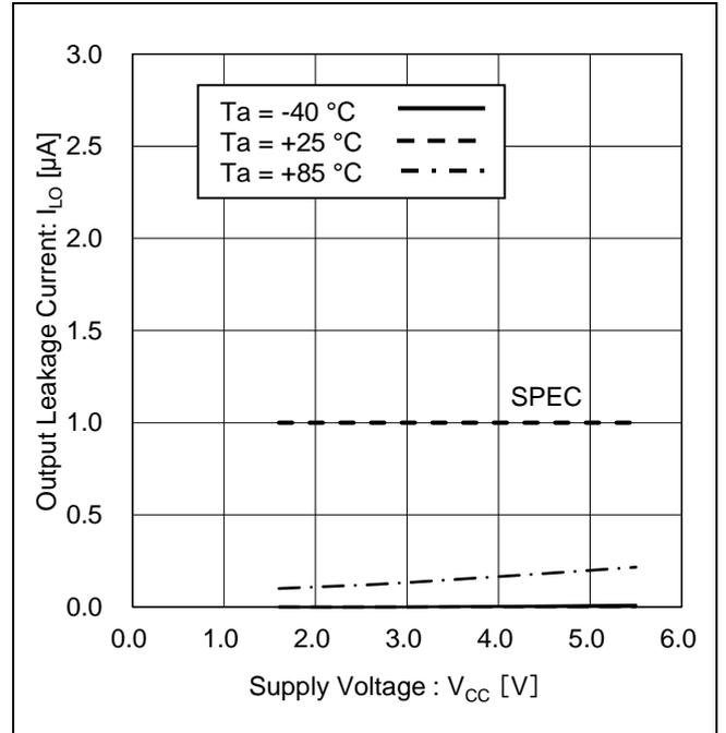
Figure 14. Output Leakage Current vs Supply Voltage (SO)
