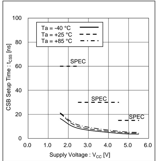
Figure 24. CSB Setup Time vs Supply Voltage
