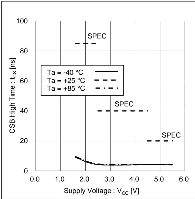
Figure 23. CSB High Time vs Supply Voltage
