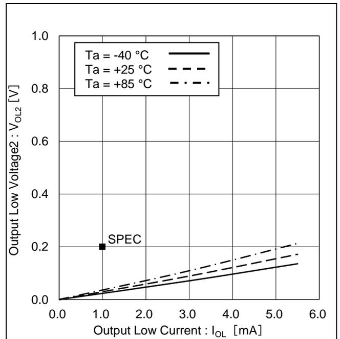
Figure 10. Output Low Voltage2 vs Output Low Current (V<sub>CC</sub> = 1.6 V)
