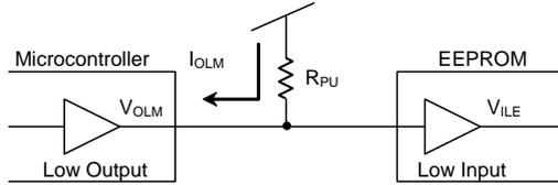
$$R_{PU} \geq \frac{V_{CC} - V_{OLM}}{I_{OLM}} \quad (1)$$
