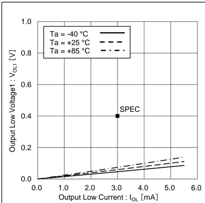
Figure 9. Output Low Voltage1 vs Output Low Current (V<sub>CC</sub> = 2.5 V)
