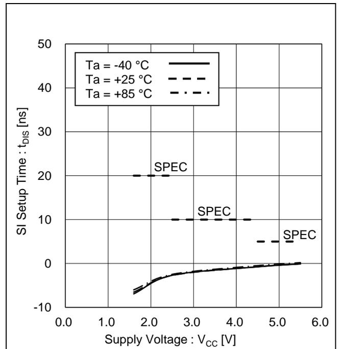
Figure 26. SI Setup Time vs Supply Voltage
