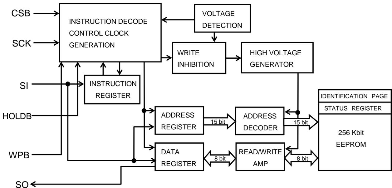
Figure 4. Block Diagram
