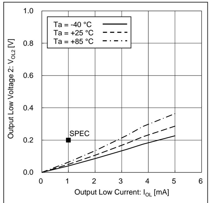
Figure 9. Output Low Voltage 2 vs Output Low Current
