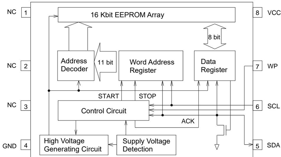
Figure 4. Block Diagram
