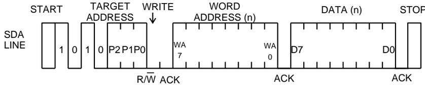
Figure 40. Byte Write
