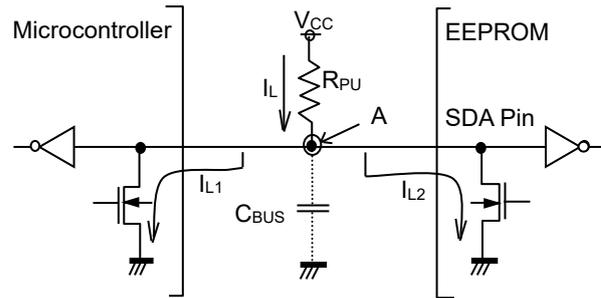
Figure 49. I/O Circuit Diagram
