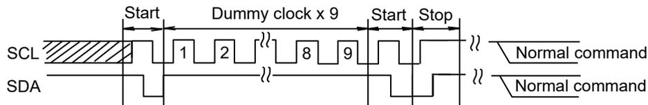
Figure 45. Input Timing of Software Reset
