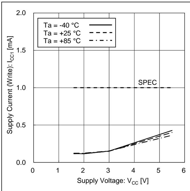
Figure 12. Supply Current (Write) vs Supply Voltage (f<sub>SCL</sub> = 1 MHz)
