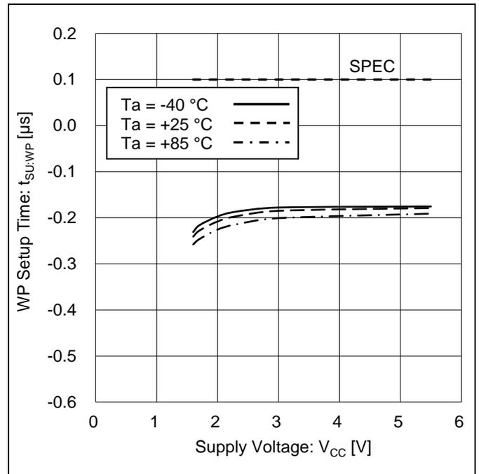
Figure 37. WP Setup Time vs Supply Voltage
