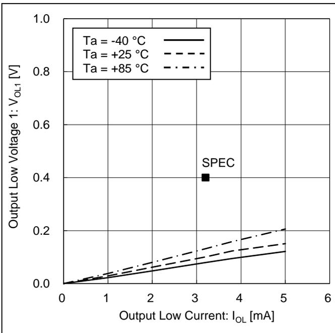
Figure 8. Output Low Voltage 1 vs Output Low Current
