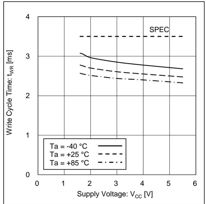
Figure 31. Write Cycle Time vs Supply Voltage
