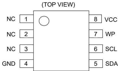
Figure 3-(a). Pin Configuration
