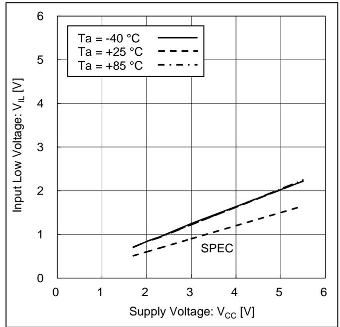
Figure 7. Input Low Voltage 1,2 vs Supply Voltage
