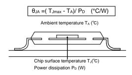
Figure 7. Thermal resistance
