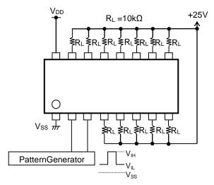
Figure 2. Test Circuit of Input H/LVoltage
