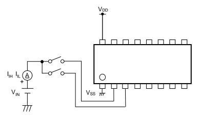
Figure 4. Test Circuit of Input H/LCurrent
