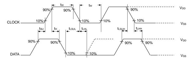
Figure 1. Waveform of Timing Characteristics
