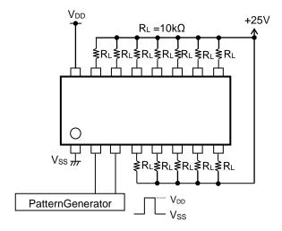
Figure 6. Test Circuit of Timing Characteristics
