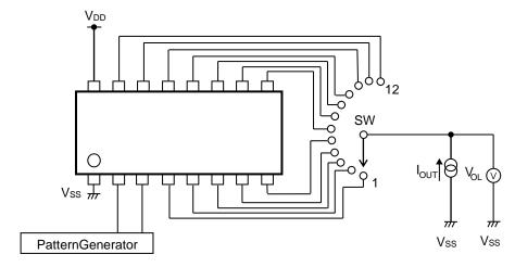
Figure 3. Test Circuit of Output L Voltage
