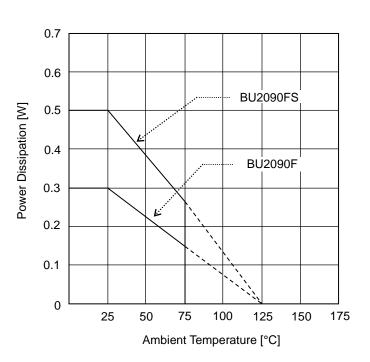
Figure 8. Derating Curve
