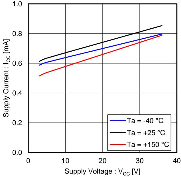
Figure 1. Supply Current vs Supply Voltage
