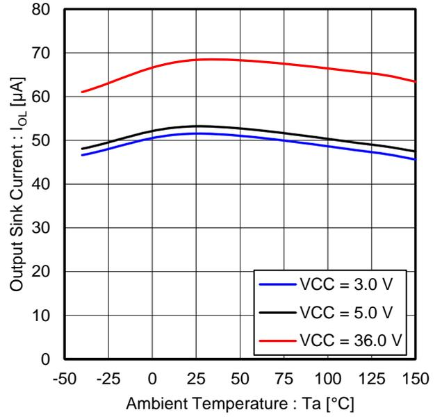
Figure 10. Output Sink Current vs Ambient Temperature
