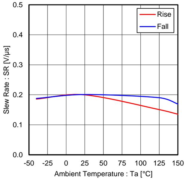
Figure 25. Slew Rate vs Ambient Temperature
