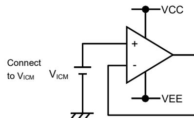
Figure 29. Example of application unused circuit processing
