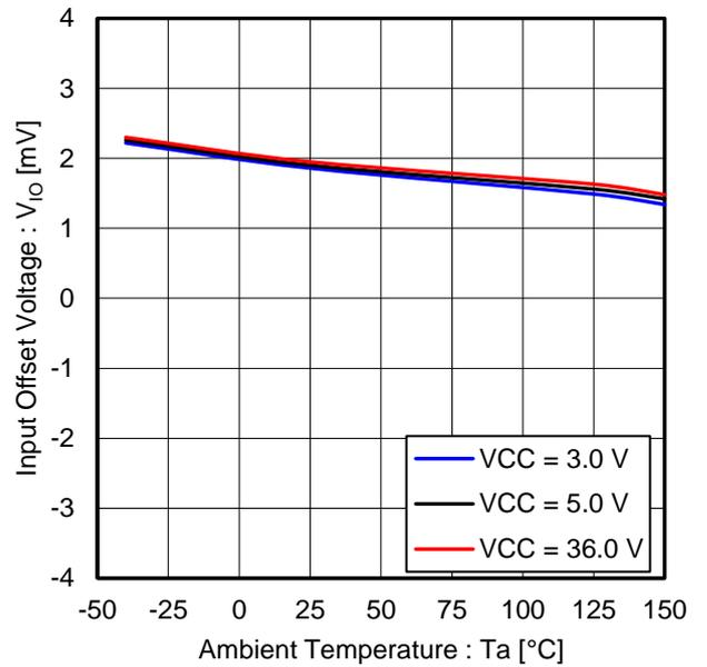
Figure 12. Input Offset Voltage vs Ambient Temperature
