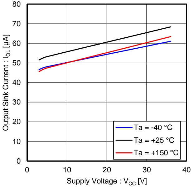
Figure 9. Output Sink Current vs Supply Voltage
