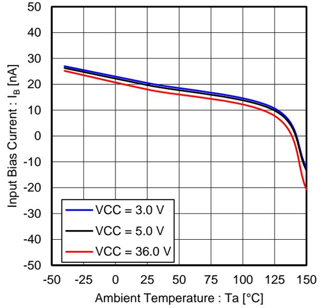
Figure 14. Input Bias Current vs Ambient Temperature
