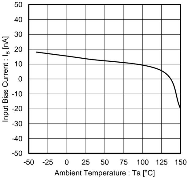
Figure 15. Input Bias Current vs Ambient Temperature
