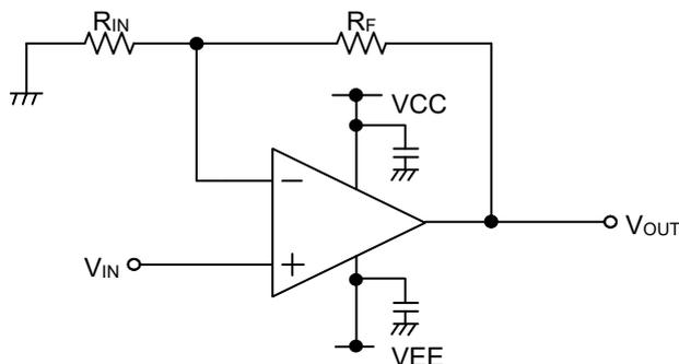
Figure 32. Non-inverting Amplifier Circuit
