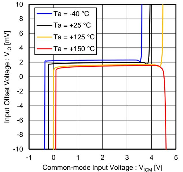
Figure 16. Input Offset Voltage vs Common-mode Input Voltage
