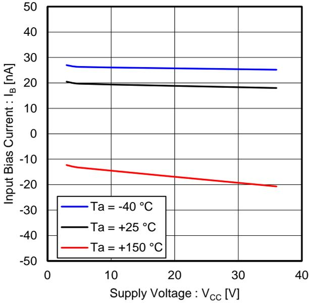
Figure 13. Input Bias Current vs Supply Voltage
