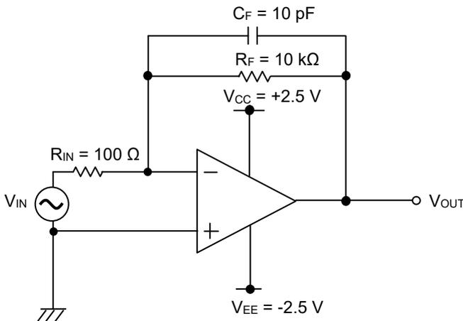
$$V_{OUT} = -\frac{R_F}{R_{IN}} V_{IN}$$
