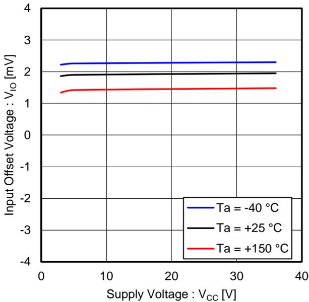
Figure 11. Input Offset Voltage vs Supply Voltage
