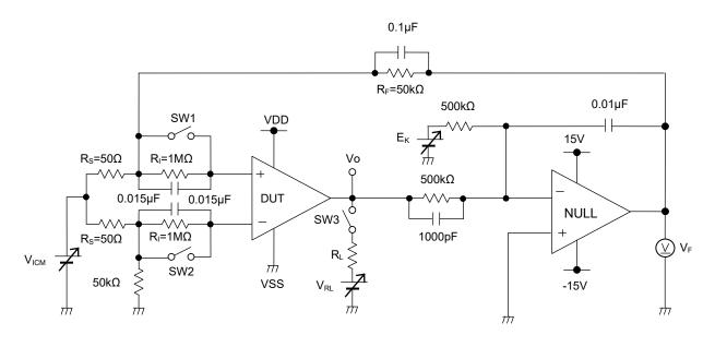
Figure 71. Test Circuit 1 (One Channel Only)
