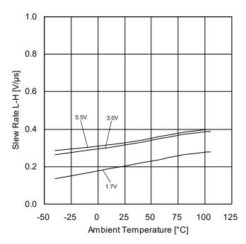
Figure 68. Slew Rate L-H vs Ambient Temperature
