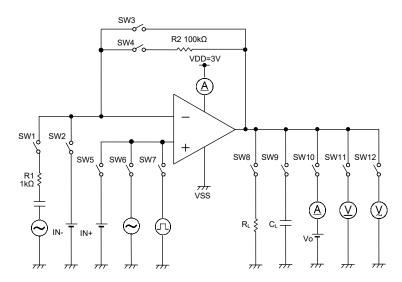
Figure 72. Test Circuit 2 (each channel)
