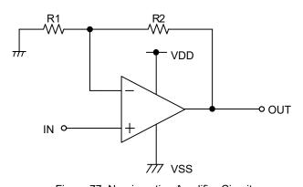
Figure 77. Non-inverting Amplifier Circuit
