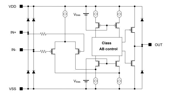
Figure 1. Simplified Schematic (1 channel only)
