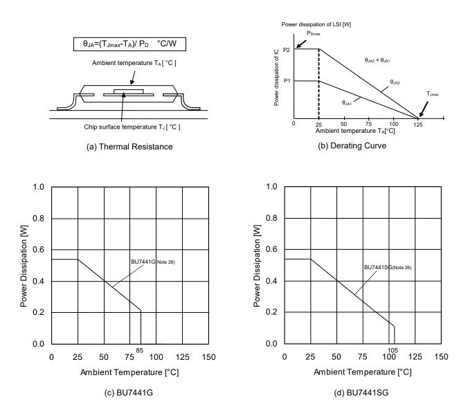
Figure 78. Thermal Resistance and Derating Curve
