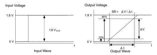
Figure 73. Slew Rate Input Output Wave
