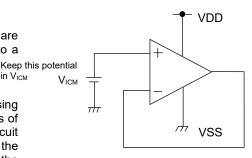
Figure 79. Example of Application Circuit for Unused Op-amp
