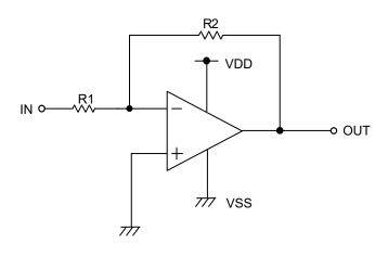
Figure 76. Inverting Amplifier Circuit
