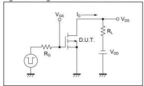
Fig.5-1 Gate Charge Measurement Circuit
