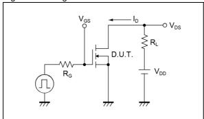
Fig.2-1 Gate Charge Measurement Circuit
