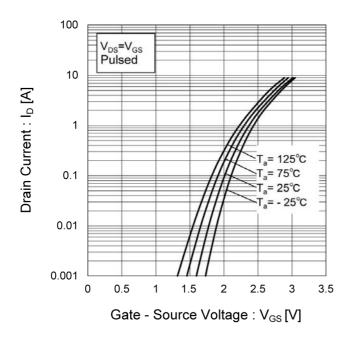
Fig.9 Gate Threshold Voltage vs.
