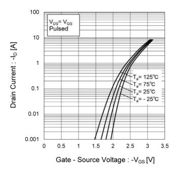
Fig.9 Gate Threshold Voltage vs.
