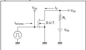
Fig.3-1 Avalanche Measurement Circuit
