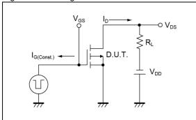
Fig.6-1 Avalanche Measurement Circuit
