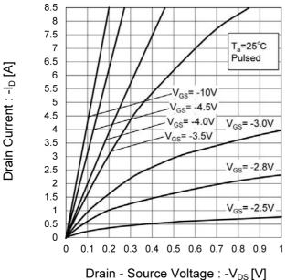
Fig.6 Typical Output Characteristics(II)
