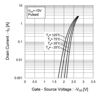
Fig.9 Gate Threshold Voltage vs.
