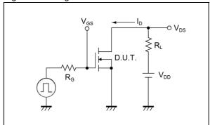
Fig.2-1 Gate Charge Measurement Circuit
