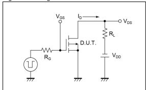
Fig.4-1 Gate Charge Measurement Circuit
