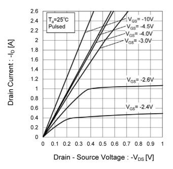
Fig.6 Typical Output Characteristics(II)
