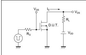
Fig.4-1 Gate Charge Measurement Circuit
