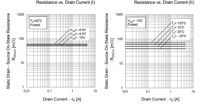
Fig.14 Static Drain - Source On - State Resistance vs. Drain Current (I)
