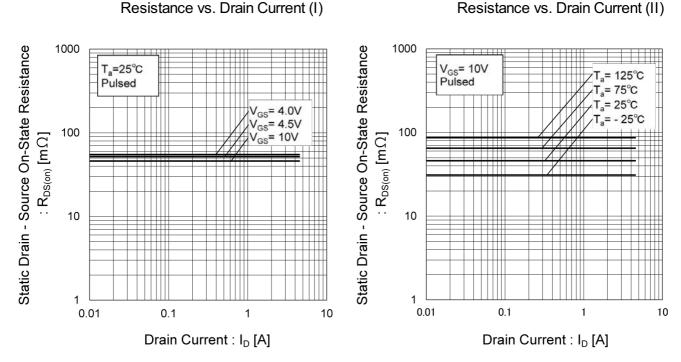
Fig.14 Static Drain - Source On - State Resistance vs. Drain Current (I)
