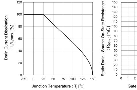
Fig.11 Drain Current Derating Curve
