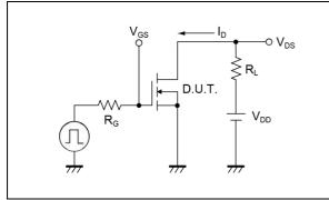
Fig.2-1 Gate Charge Measurement Circuit
