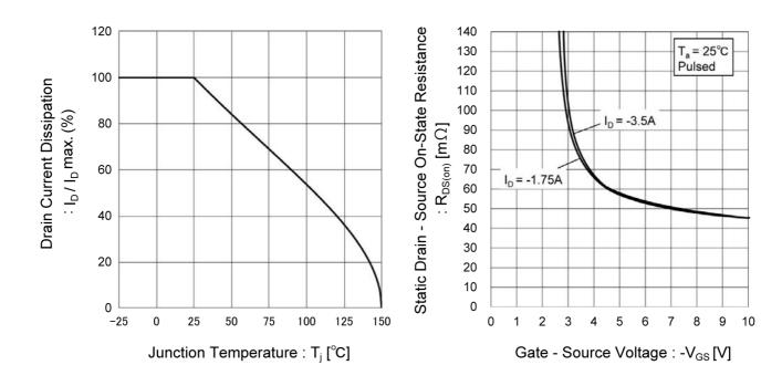
Fig.11 Drain Current Derating Curve
