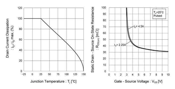
Fig.11 Drain Current Derating Curve
