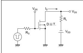
Fig.4-1 Gate Charge Measurement Circuit
