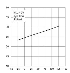
Fig.7 Breakdown Voltage vs. Junction
