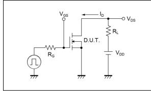
Fig.2-1 Gate Charge Measurement Circuit
