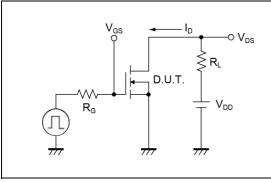
Fig.2-1 Gate Charge Measurement Circuit
