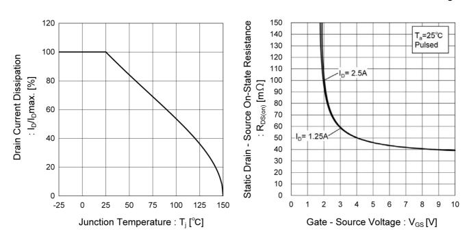
Fig.11 Drain Current Derating Curve
