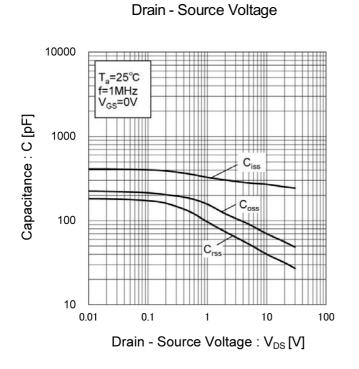
Fig.18 Typical Capacitance vs.
