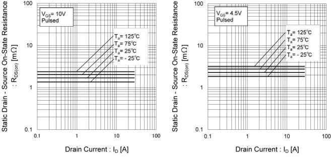
Fig.14 Static Drain - Source On - State Resistance vs. Drain Current(I)
