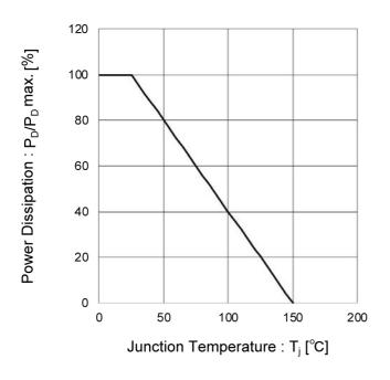
Fig.1 Power Dissipation Derating Curve
