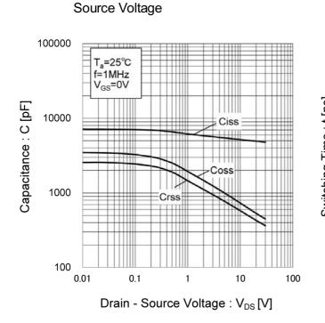
Fig.17 Typical Capacitance vs. Drain -
