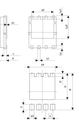
Pattern of terminal position areas [Not a pattern of soldering pads]
