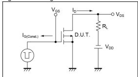
Fig.3-1 Avalanche Measurement Circuit
