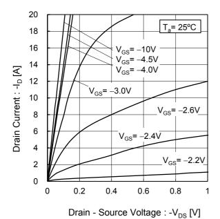
Fig.8 Typical Output Characteristics(II)
