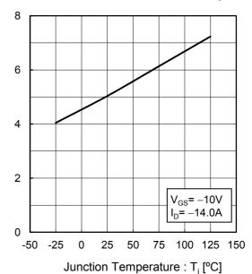
Static Drain - Source On-State Resistance
