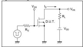
Fig.2-1 Gate Charge Measurement Circuit
