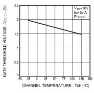
Fig.9 Gate Threshold Voltage vs. Channel Temperature
