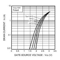
Fig.3 Typical Transfer Characteristics
