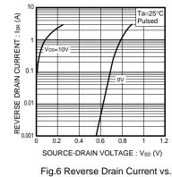
ig.6 Reverse Drain Current vs. Source-Drain Voltage ( II )
