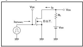
Fig.3-1 Avalanche Measurement Circuit
