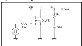
Fig.2-1 Gate Charge Measurement Circuit
