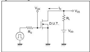
Fig.2-1 Gate Charge Measurement Circuit
