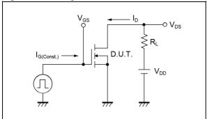
Fig.3-1 Avalanche Measurement Circuit
