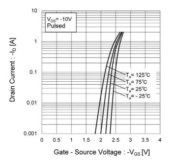
Fig.9 Gate Threshold Voltage vs.
