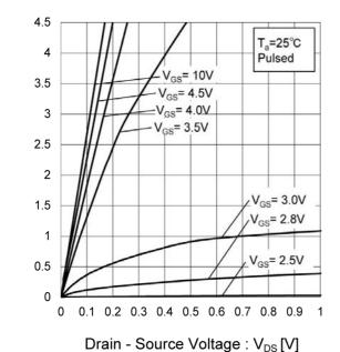
Fig.6 Typical Output Characteristics(II)
