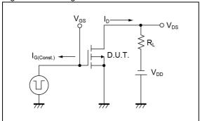
Fig.6-1 Avalanche Measurement Circuit
