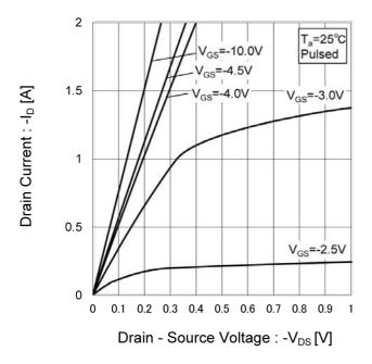
Fig.6 Typical Output Characteristics(II)
