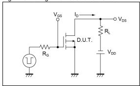
Fig.5-1 Gate Charge Measurement Circuit
