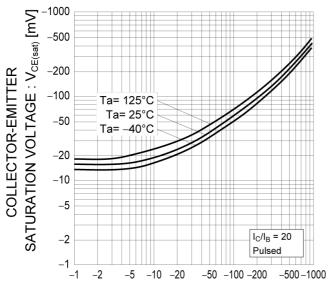
Fig.6 Collector-Emitter Saturation
