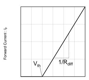
Fig.11 Equivalent forward current curve
