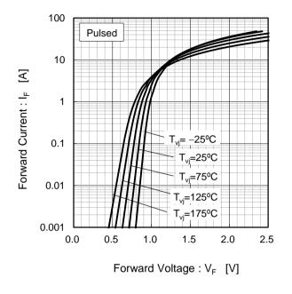
Fig.1 V<sub>F</sub> - I<sub>F</sub> Characteristics
