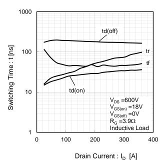
Fig.11 Switching Characteristics [T<sub>i</sub>=150°C]
