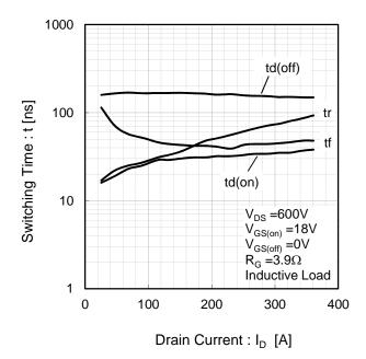
Fig.10 Switching Characteristics [T<sub>i</sub>=125°C]
