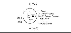
Please note Driver Source and Power Source are not exchangeable. Their exchange might lead to malfunction.
