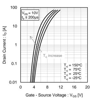
Fig.9 Typical Transfer Characteristics (I)
