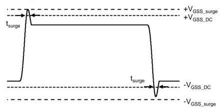
Please note especially when using driver source that  $V_{GSS\_surge}$  must be in the range of absolute maximum rating.
