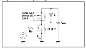
Fig.4-1 Reverse Recovery Time Measurement Circuit Fig.4-2 Reverse Recovery Waveform
