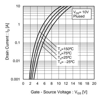
Fig.9 Typical Transfer Characteristics (II)
