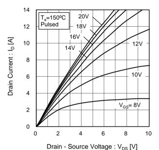
Fig.7 T<sub>j</sub> = 150°C Typical Output Characteristics(II)
