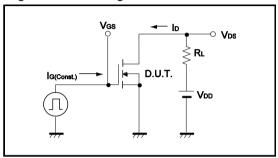
Fig.3-1 Switching Energy Measurement Circuit
