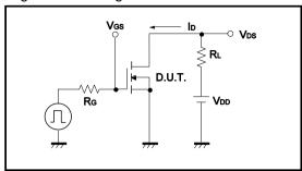
Fig.2-1 Gate Charge Measurement Circuit
